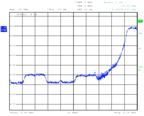
Figure 25 Plot of Transmitter Low Band Edge Chain 1 (5150-5250 MHz Band, 802.11a)
