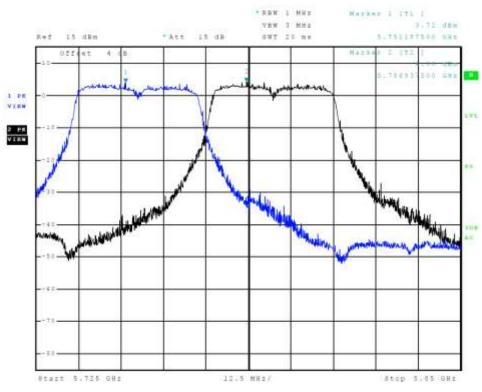
Figure 34 Plot of Transmitter Emissions Chain 1 (Across 5725-5850 MHz Band, 802.11n40)
