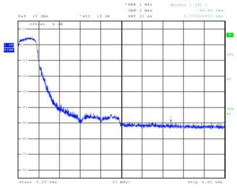
Figure 8 Plot of Transmitter High Band Edge Chain 0 (5150-5250 MHz Band, 802.11n40)
