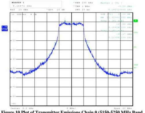
Figure 10 Plot of Transmitter Emissions Chain 0 (5150-5250 MHz Band, 802.11a, 26 dB OBW)
