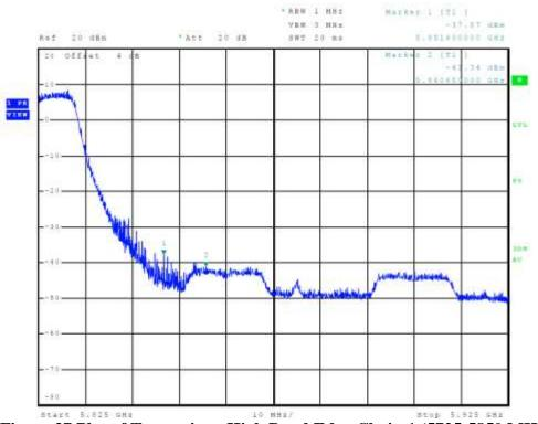
Figure 37 Plot of Transmitter High Band Edge Chain 1 (5725-5850 MHz Band, 802.11a)
