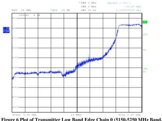
Figure 6 Plot of Transmitter Low Band Edge Chain 0 (5150-5250 MHz Band, 802.11n40)
