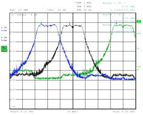
Figure 3 Plot of Transmitter Emissions Chain 0 (Across 5150-5250 MHz Band, 802.11a)
