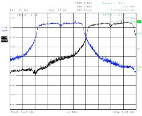
Figure 24 Plot of Transmitter Emissions Chain 1 (Across 5150-5250 MHz Band, 802.11n40)
