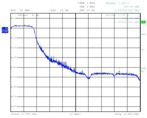
Figure 38 Plot of Transmitter High Band Edge Chain 1 (5725-5850 MHz Band, 802.11n40)
