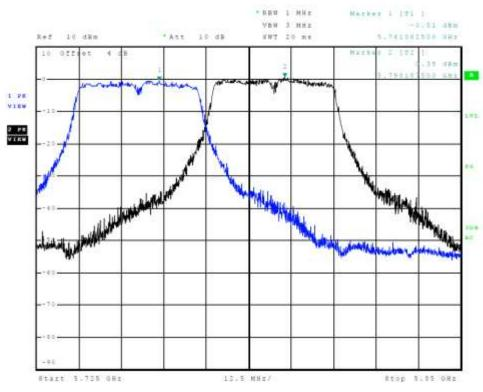
Figure 14 Plot of Transmitter Emissions Chain 0 (Across 5725-5850 MHz Band, 802.11n40)
