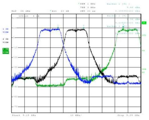
Figure 23 Plot of Transmitter Emissions Chain 1 (Across 5150-5250 MHz Band, 802.11a)
