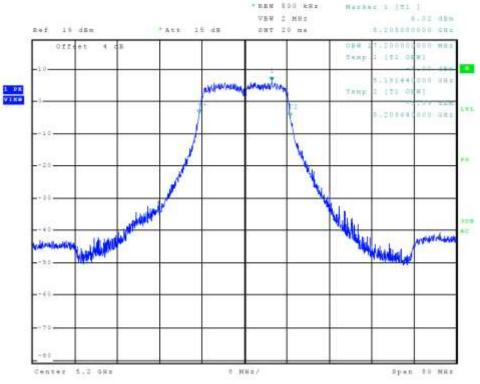
Figure 29 Plot of Transmitter Emissions Chain 1 (5150-5250 MHz Band, 802.11a, 99% OBW)
