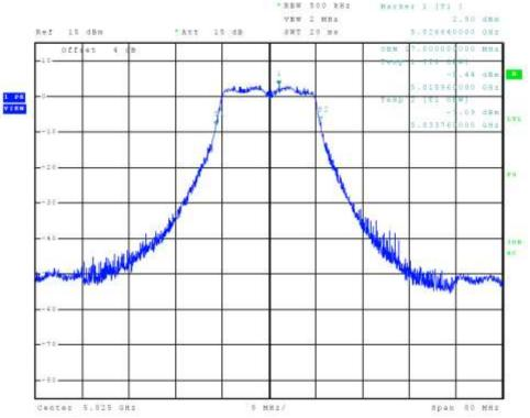
Figure 19 Plot of Transmitter Emissions Chain 0 (5725-5850 MHz Band, 802.11a, 99% OBW)
