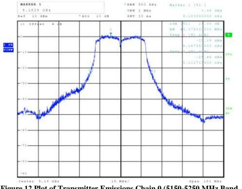
Figure 12 Plot of Transmitter Emissions Chain 0 (5150-5250 MHz Band, 802.11n40, 26 dB OBW)
