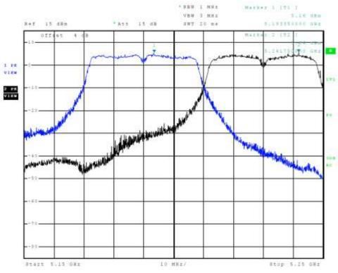
Figure 4 Plot of Transmitter Emissions Chain 0 (Across 5150-5250 MHz Band, 802.11n40)
