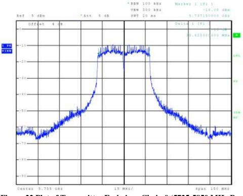
Figure 22 Plot of Transmitter Emissions Chain 0 (5725-5850 MHz Band, 802.11n40, 6-dB OBW)
