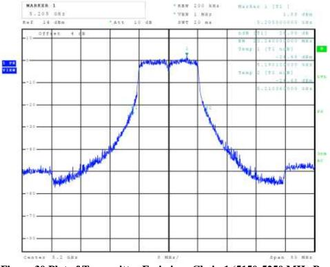
Figure 30 Plot of Transmitter Emissions Chain 1 (5150-5250 MHz Band, 802.11a, 26 dB OBW)
