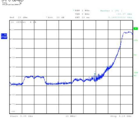
Figure 5 Plot of Transmitter Low Band Edge Chain 0 (5150-5250 MHz Band, 802.11a)
