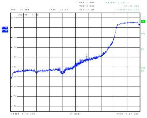
Figure 26 Plot of Transmitter Low Band Edge Chain 1 (5150-5250 MHz Band, 802.11n40)
