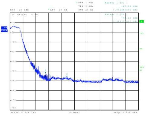
Figure 17 Plot of Transmitter High Band Edge Chain 0 (5725-5850 MHz Band, 802.11a)
