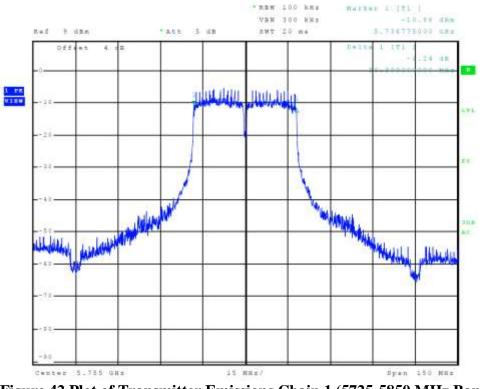
Figure 42 Plot of Transmitter Emissions Chain 1 (5725-5850 MHz Band, 802.11n40, 6-dB OBW)
