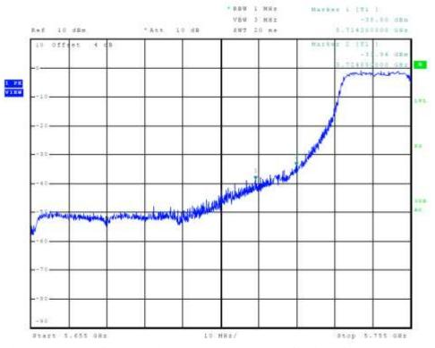
Figure 16 Plot of Transmitter Low Band Edge Chain 0 (5725-5850 MHz Band, 802.11n40)
