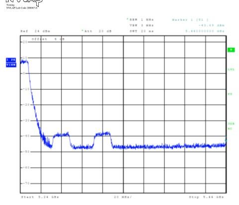
Figure 27 Plot of Transmitter High Band Edge Chain 1 (5150-5250 MHz Band, 802.11a)
