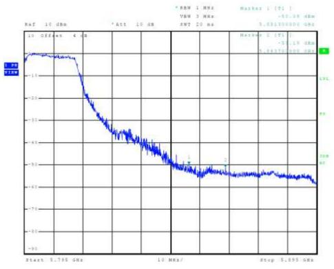
Figure 18 Plot of Transmitter High Band Edge Chain 0 (5725-5850 MHz Band, 802.11n40)
