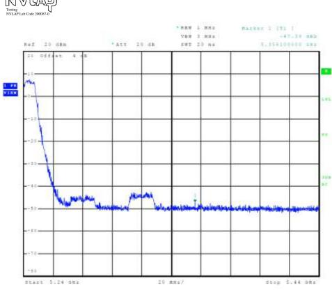
Figure 7 Plot of Transmitter High Band Edge Chain 0 (5150-5250 MHz Band, 802.11a)
