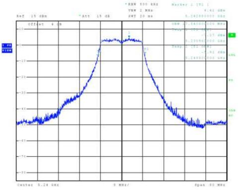
Figure 9 Plot of Transmitter Emissions Chain 0 (5150-5250 MHz Band, 802.11a, 99% OBW)
