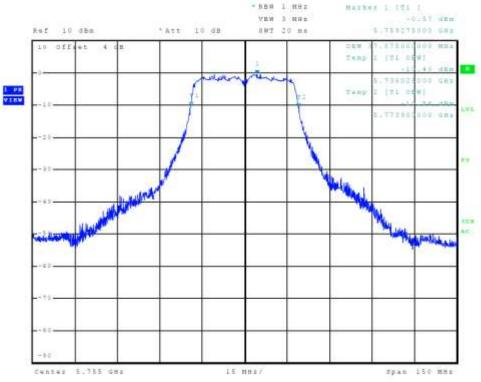
Figure 21 Plot of Transmitter Emissions Chain 0 (5725-5850 MHz Band, 802.11n40, 99% OBW)
