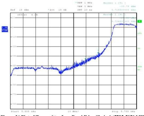
Figure 36 Plot of Transmitter Low Band Edge Chain 1 (5725-5850 MHz Band, 802.11n40)
