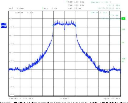
Figure 20 Plot of Transmitter Emissions Chain 0 (5725-5850 MHz Band, 802.11a, 6-dB OBW)
