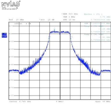
Figure 39 Plot of Transmitter Emissions Chain 1 (5725-5850 MHz Band, 802.11a, 99% OBW)
