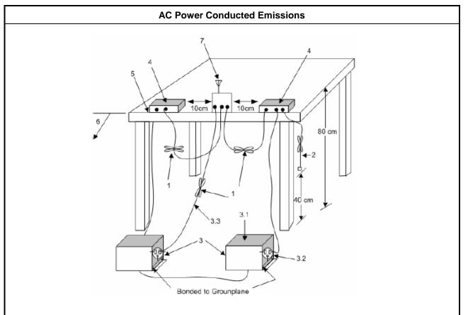
1—Interconnecting cables that hang closer than 40 cm to the ground plane shall be folded back and forth in the center forming a bundle 30 cm to 40 cm long.
