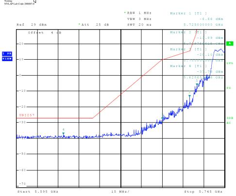
Figure 27 Plot of Transmitter Low Band Edge (5725-5850 MHz Band, Chain 0, 802.11a)
