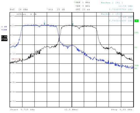
Figure 26 Plot of Transmitter Emissions (Across 5725-5850 MHz Band, Chain 1, 802.11n40)
