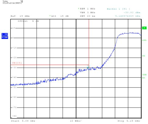
Figure 9 Plot of Transmitter Low Band Edge (5150-5250 MHz Band, Chain 0, 802.11n40)
