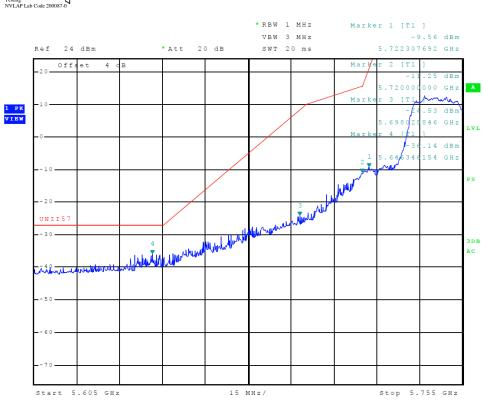
Figure 29 Plot of Transmitter Low Band Edge (5725-5850 MHz Band, Chain 0, 802.11n40)
