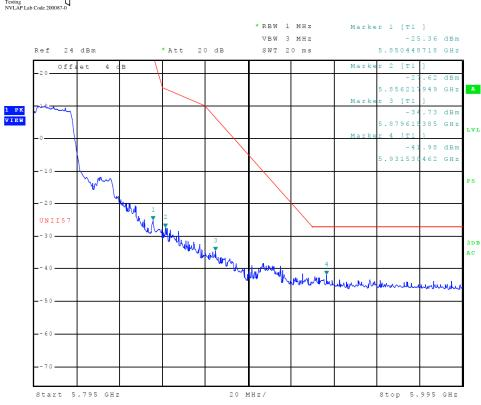
Figure 33 Plot of Transmitter High Band Edge (5725-5850 MHz Band, Chain 0, 802.11n40)
