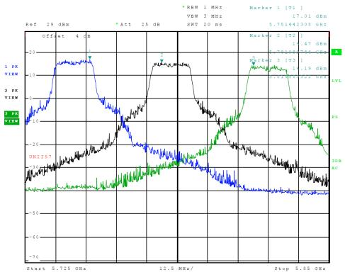
Figure 24 Plot of Transmitter Emissions (Across 5725-5850 MHz Band, Chain 1, 802.11a)
