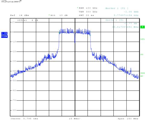
Figure 41 Plot of Transmitter Emissions (5725-5850 MHz Band, 802.11n40, Chain 0, 6-dB OBW)
