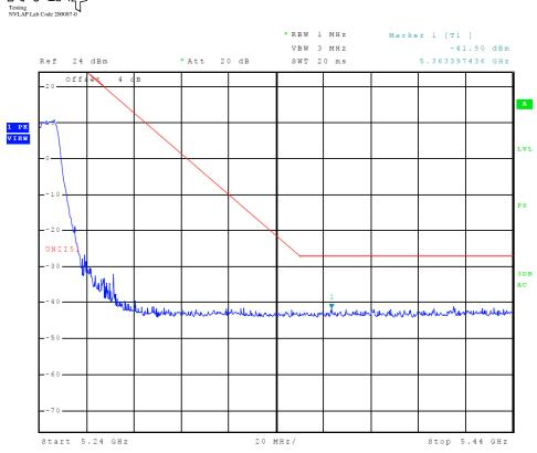
Figure 11 Plot of Transmitter High Band Edge (5150-5250 MHz Band, Chain 0, 802.11a)
