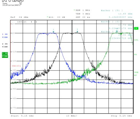
Figure 3 Plot of Transmitter Emissions (Across 5150-5250 MHz Band, Chain 0, 802.11a)
