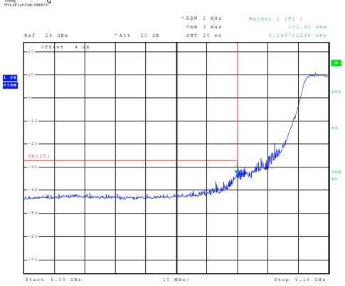
Figure 7 Plot of Transmitter Low Band Edge (5150-5250 MHz Band, Chain 0, 802.11a)
