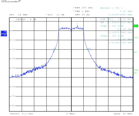
Figure 17 Plot of Transmitter Emissions (5150-5250 MHz Band, 802.11a, Chain 0, 26 dB OBW)
