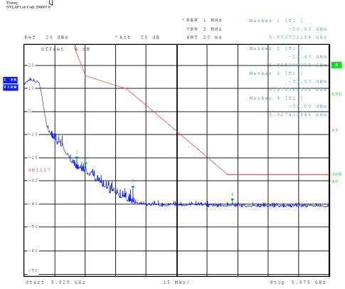
Figure 31 Plot of Transmitter High Band Edge (5725-5850 MHz Band, Chain 0, 802.11a)
