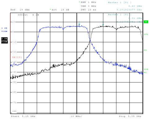
Figure 6 Plot of Transmitter Emissions (Across 5150-5250 MHz Band, Chain 1, 802.11n40)
