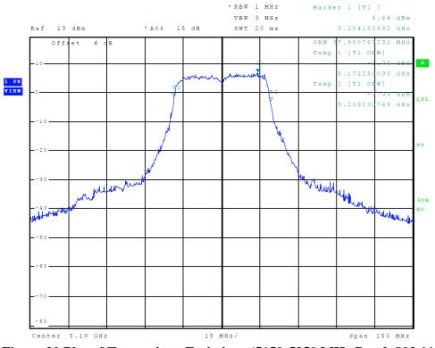
Figure 20 Plot of Transmitter Emissions (5150-5250 MHz Band, 802.11n40, Chain 1, 99% OBW)
