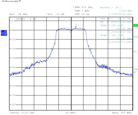
Figure 21 Plot of Transmitter Emissions (5150-5250 MHz Band, 802.11n40, Chain 0, 26 dB OBW)
