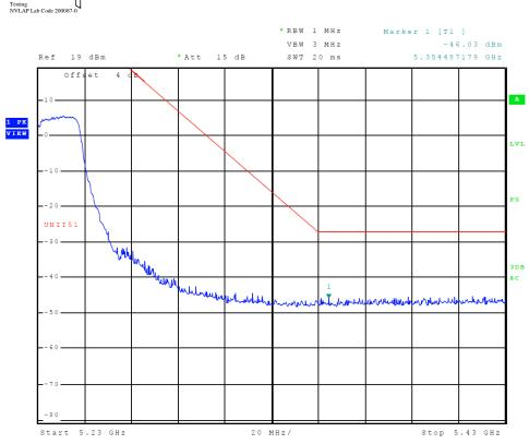
Figure 13 Plot of Transmitter High Band Edge (5150-5250 MHz Band, Chain 0, 802.11n40)
