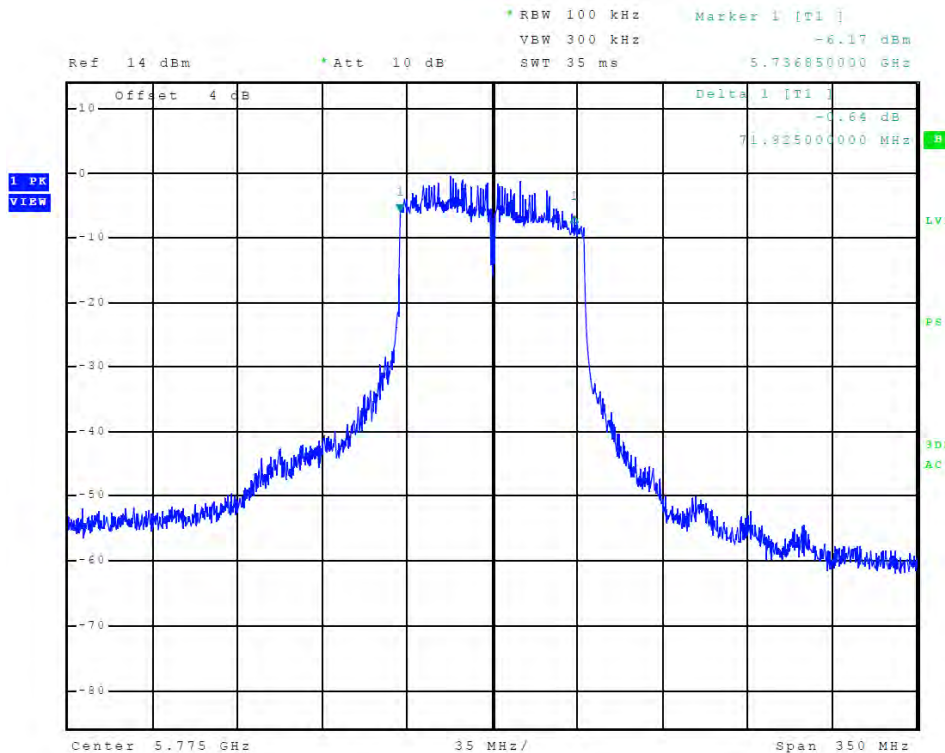
Figure 90 Plot of Chain 0 Emissions (5725-5850 MHz Band, 802.11ac, 6-dB OBW)
