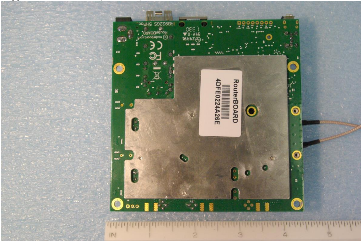
Support interface board (back side)
