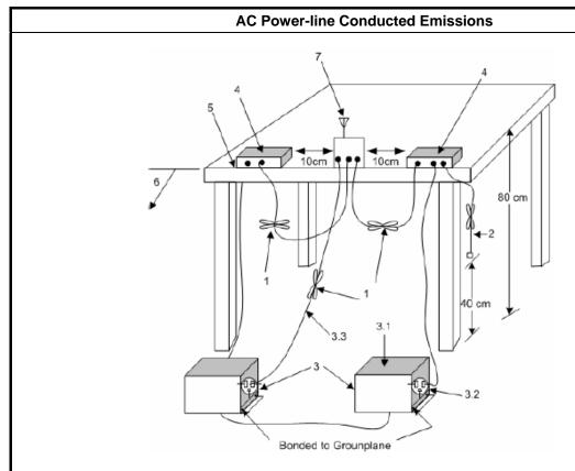
1—Interconnecting cables that hang closer than 40 cm to the ground plane shall be folded back and forth in the center forming a bundle 30 cm to 40 cm long.
