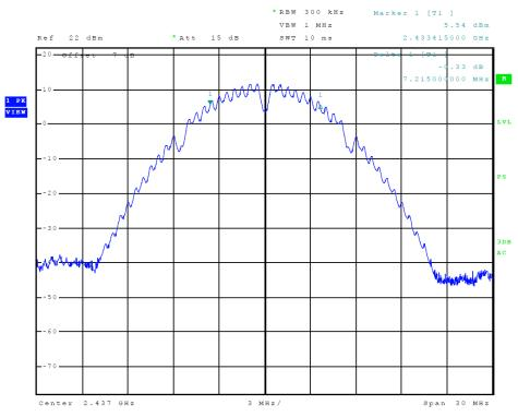
Figure 15 Plot of Transmitter 6-dB Occupied Band Width (802.11b)
