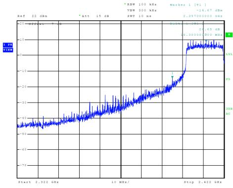
Figure 10 Plot of Transmitter Low Band Edge (802.11n (40))
