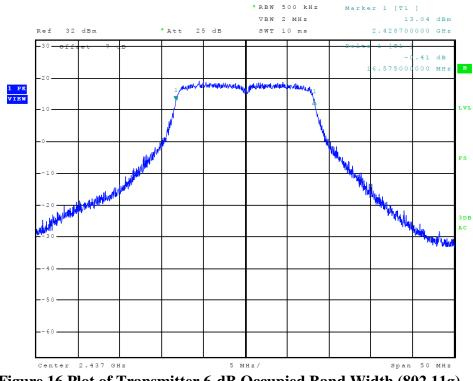
Figure 16 Plot of Transmitter 6-dB Occupied Band Width (802.11g)
