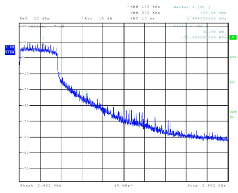
Figure 14 Plot of Transmitter High Band Edge (802.11n (40))
