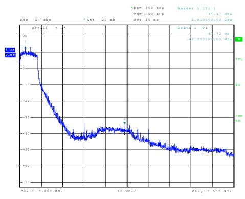
Figure 12 Plot of Transmitter High Band Edge (802.11g)
