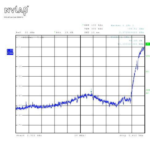
Figure 7 Plot of Transmitter Low Band Edge (802.11b)
