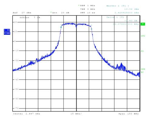
Figure 18 Plot of Transmitter 6-dB Occupied Band Width (802.11n (40))
