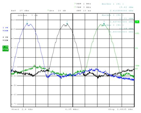
Figure 3 Plot of Transmitter Emissions (Across Operational Band 802.11b)
