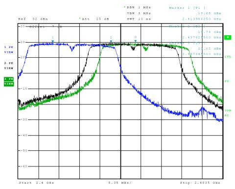
Figure 6 Plot of Transmitter Emissions (Across Operational Band, 802.11n (40)
