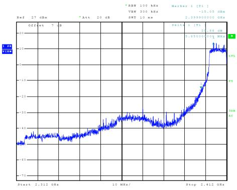
Figure 9 Plot of Transmitter Low Band Edge (802.11n (20))
