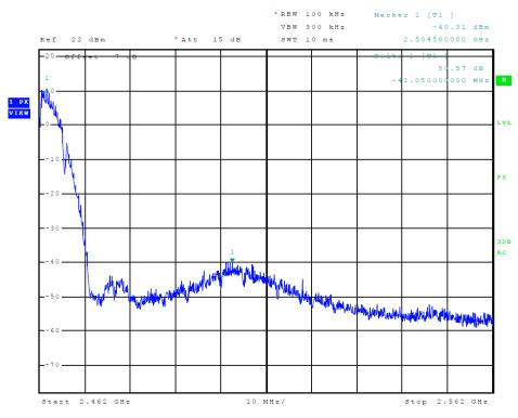
Figure 11 Plot of Transmitter High Band Edge (802.11b)
