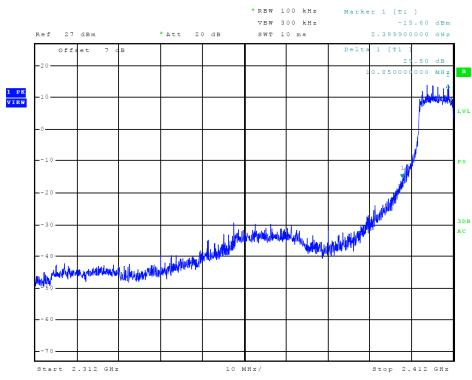
Figure 8 Plot of Transmitter Low Band Edge (802.11g)
