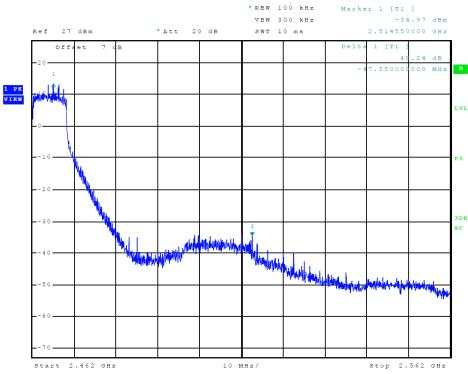
Figure 13 Plot of Transmitter High Band Edge (802.11n (20))
