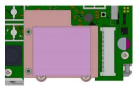
• Install module to the miniPCIe slot and secure with previously removed screws. Tightening torque 0,3 Nm.
