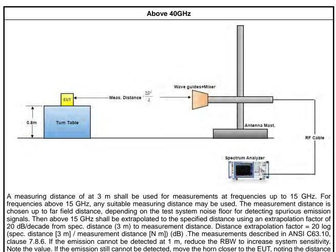
at which a measurement is made.
