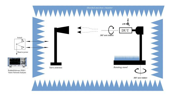
Explanation: Antenna testing is performed using the test setup above. Antenna gain is measured in 3d plane. The measurments are then taken and ran through CST studio Time domain solver sumulation system to draw Antenna peak gain diagram. Simulation is performed taking into account pcb with components, case desing, heatsink and etc.
