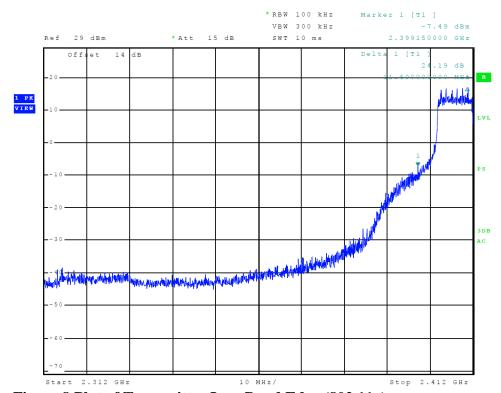
Figure 8 Plot of Transmitter Low Band Edge (802.11g)
