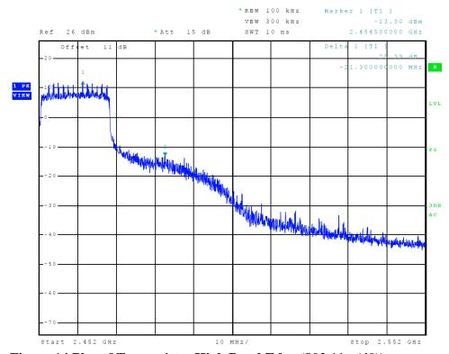
Figure 14 Plot of Transmitter High Band Edge (802.11n (40))
