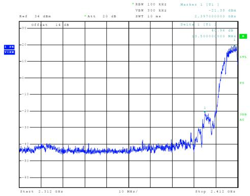
Figure 7 Plot of Transmitter Low Band Edge (802.11b)
