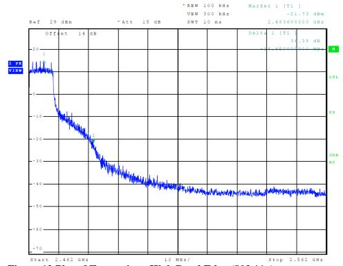
Figure 12 Plot of Transmitter High Band Edge (802.11g)
