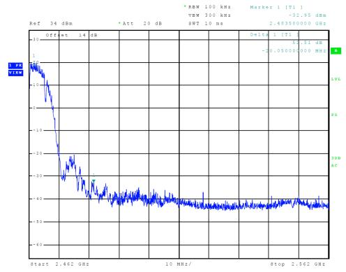
Figure 11 Plot of Transmitter High Band Edge (802.11b)
