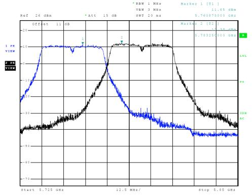
Figure 14 Plot of Transmitter Emissions (Across 5725-5850 MHz Band, 802.11n40)
