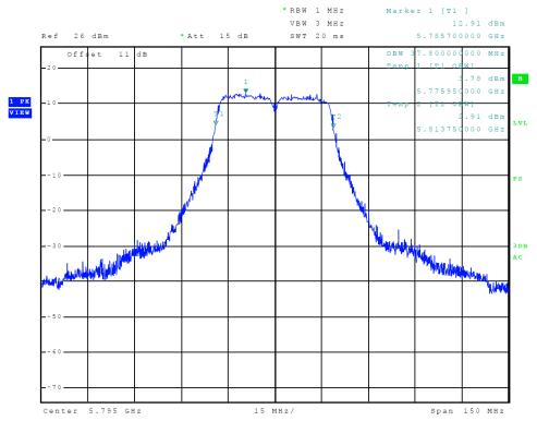
Figure 21 Plot of Transmitter Emissions (5725-5850 MHz Band, 802.11n40, 99% OBW)
