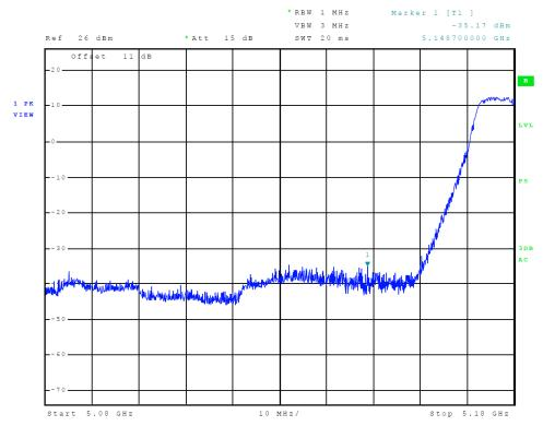
Figure 5 Plot of Transmitter Low Band Edge (5150-5250 MHz Band, 802.11a)
