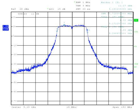
Figure 11 Plot of Transmitter Emissions (5150-5250 MHz Band, 802.11n40, 99% OBW)
