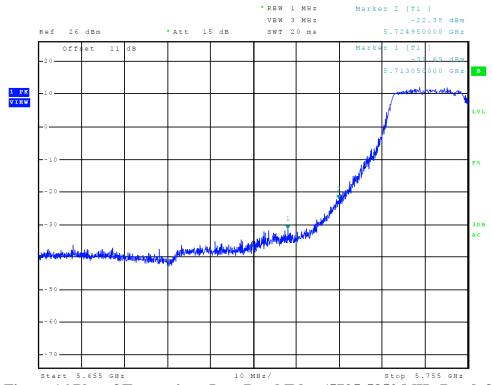
Figure 16 Plot of Transmitter Low Band Edge (5725-5850 MHz Band, 802.11n40)
