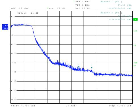
Figure 18 Plot of Transmitter High Band Edge (5725-5850 MHz Band, 802.11n40)
