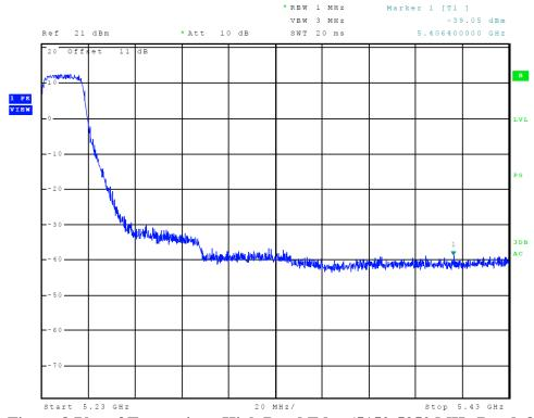
Figure 8 Plot of Transmitter High Band Edge (5150-5250 MHz Band, 802.11n40)
