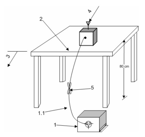
1. A LISN is optional for radiated measurements between 30 MHz to 1000 MHz, but not allowed for measurements below 30 MHz and above 1000 MHz (See 6.4.3, 6.5.1, and 6.6.3). If used, connect EUT to one LISN. Unused LISN measuring port connectors shall be terminated in  $50\Omega$ . LISN can be placed on top of, or immediately beneath, reference ground plane (see 6.2.2 and 6.2.3.1).
