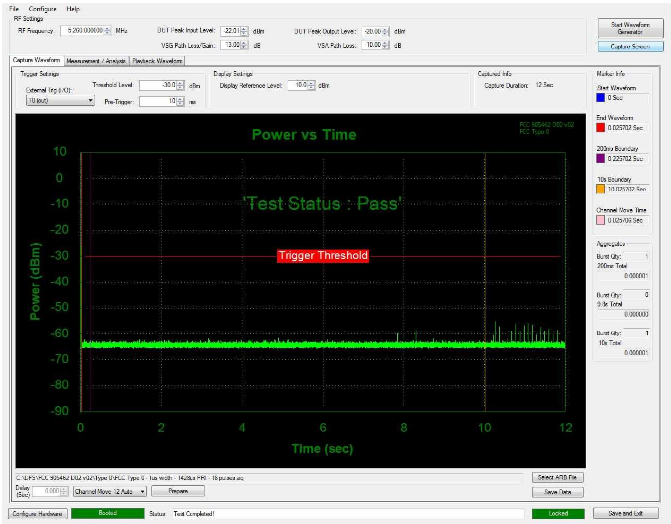
Figure 8.6-1: Channel closing transmission and move time
