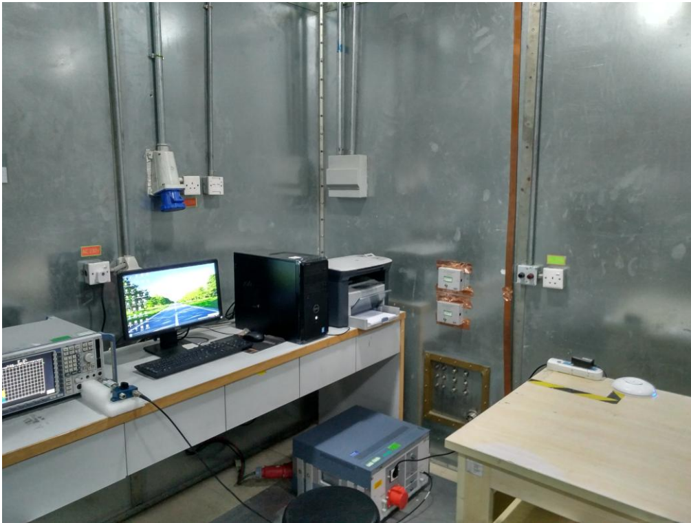
FCC RADIATED EMISSION TEST SETUP BELOW 1GHZ
