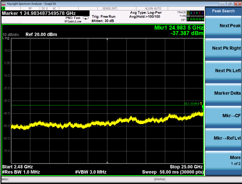
TEST PLOT OF OUT OF BAND EMISSIONS THE WORST CASE OF 802.11n40 FOR MODULATION IN MIDDLE CHANNEL
