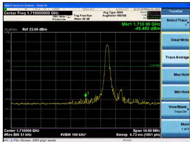
LTE Band 66 16QAM 20MHz CH-Low, 1 RB
