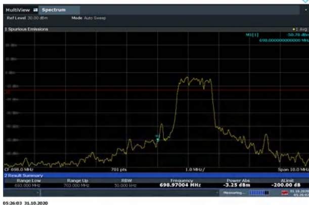
LTE Band 85 16QAM 5MHz CH-Low, 1 RB
