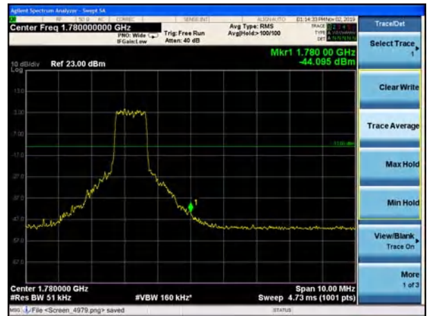
LTE Band 85 QPSK 5MHz CH-High, 1 RB
