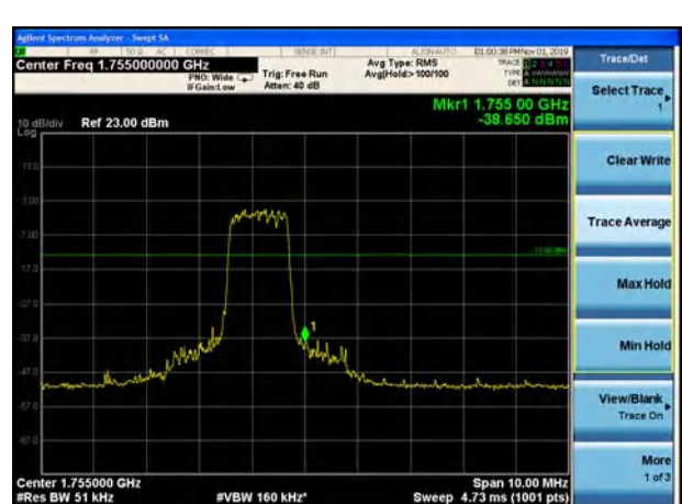
LTE Band 4 QPSK 3MHz CH-High, 100%RB
