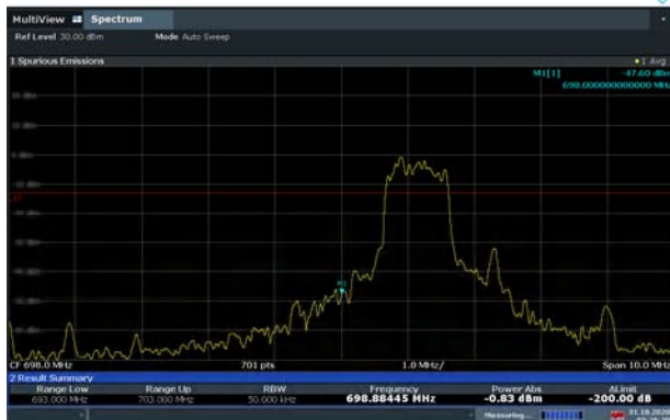
LTE Band 85 16QAM 10MHz CH-Low, 100%RB
