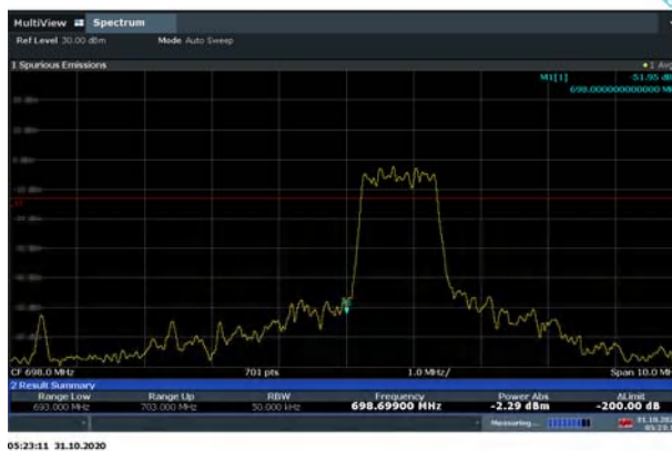
LTE Band 85 QPSK 5MHz CH-Low, 100%RB
