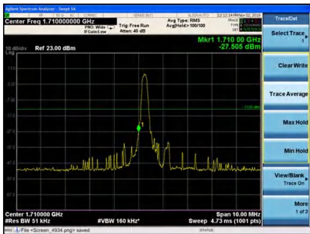
LTE Band 66 16QAM 1.4MHz CH-Low, 100%RB
