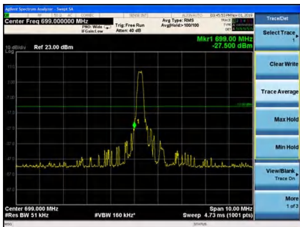
LTE Band 12 16QAM 1.4MHz CH-Low, 1 RB
