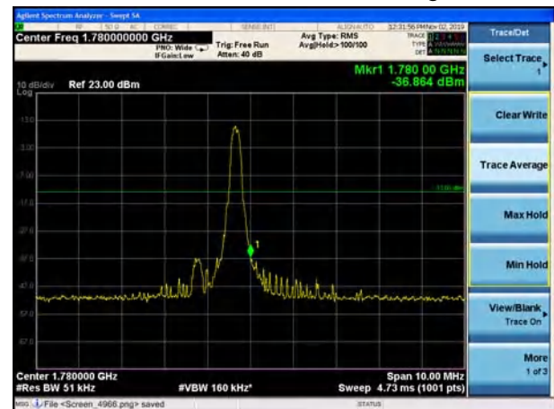
LTE Band 66 16QAM 5MHz CH-High, 1 RB
