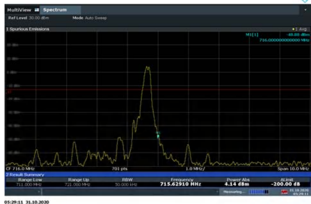
LTE Band 85 16QAM 5MHz CH-High, 1 RB
