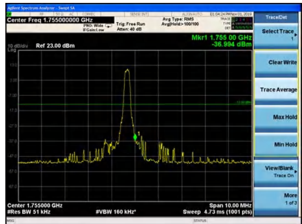
LTE Band 4 16QAM 5MHz CH-High, 100%RB
