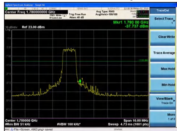
LTE Band 66 16QAM 5MHz CH-High, 1 RB
