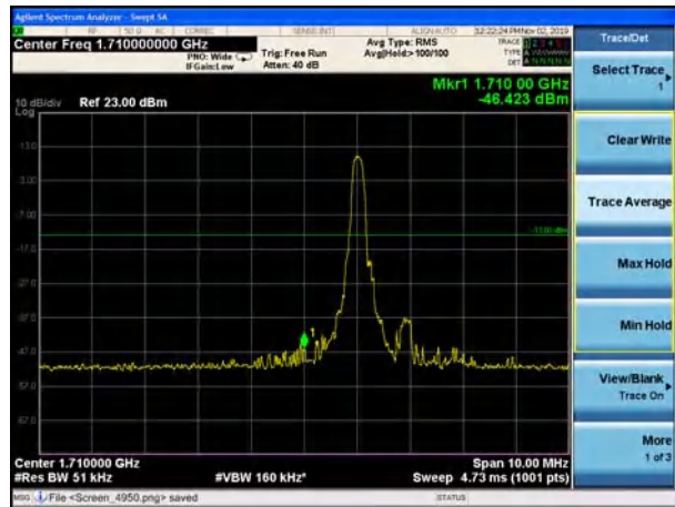
LTE Band 66 16QAM 15MHz CH-Low, 100%RB
