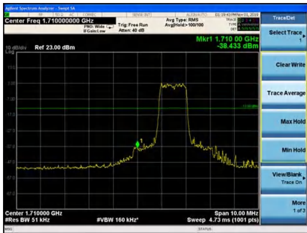
LTE Band 4 QPSK 20MHz CH-Low, 1 RB
