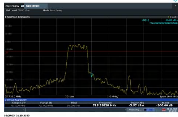
LTE Band 85 QPSK 5MHz CH-High, 100%RB
