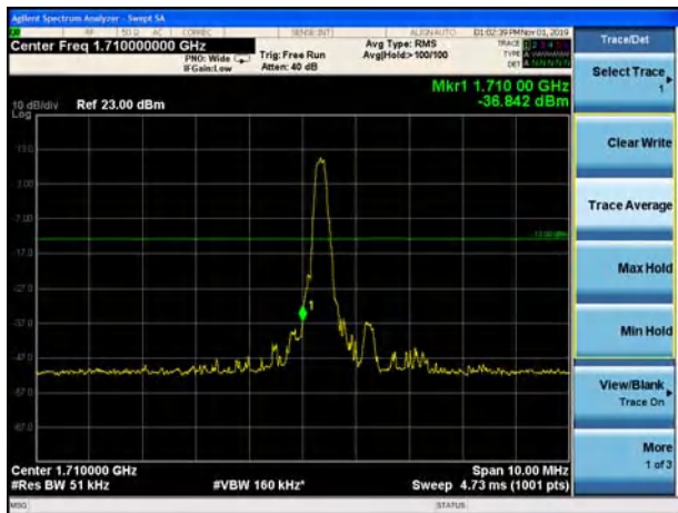
LTE Band 4 16QAM 5MHz CH-Low, 100%RB
