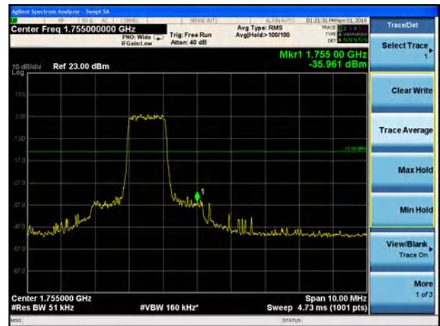
LTE Band 4 QPSK 20MHz CH-High, 1 RB
