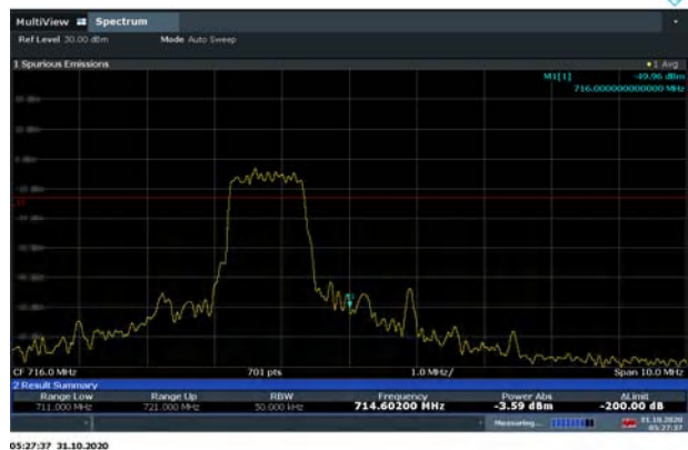
LTE Band 85 16QAM 5MHz CH-High, 1 RB
