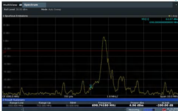
LTE Band 85 16QAM 10MHz CH-Low, 100%RB
