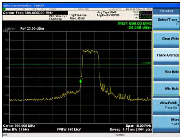
LTE Band 12 QPSK 3MHz CH-Low, 1 RB
