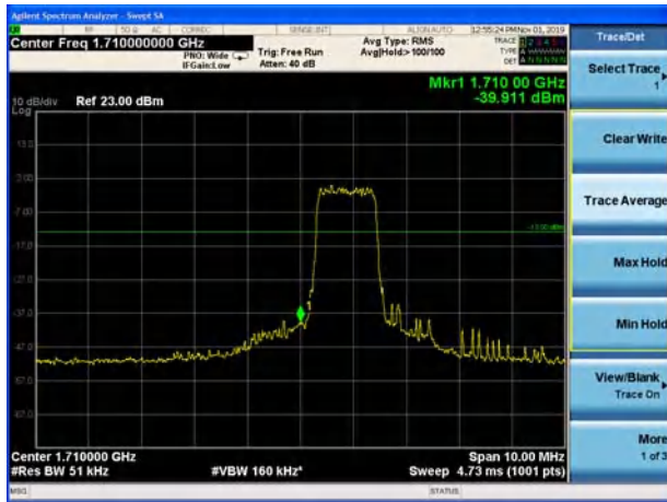
LTE Band 4 QPSK 3MHz CH-Low, 100%RB
