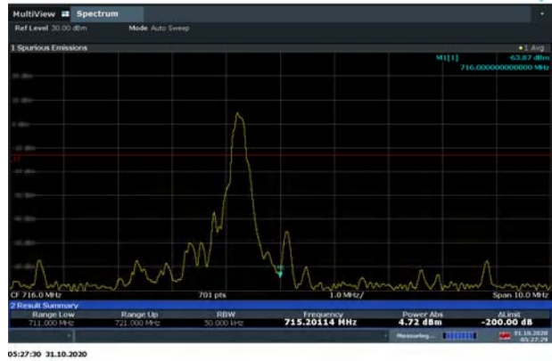
LTE Band 85 QPSK 10MHz CH-High, 100%RB
