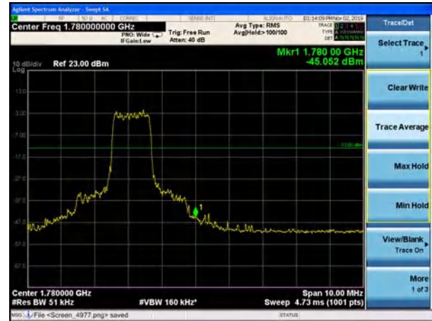
LTE Band 66 16QAM 1.4MHz CH-High, 1 RB
