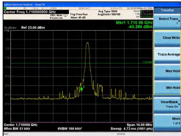
LTE Band 66 16QAM 3MHz CH-Low, 100%RB
