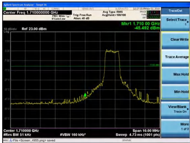
LTE Band 85 QPSK 5MHz CH-Low, 1 RB
