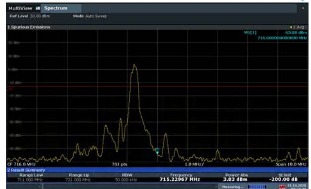
LTE Band 85 16QAM 10MHz CH-High, 100%RB
