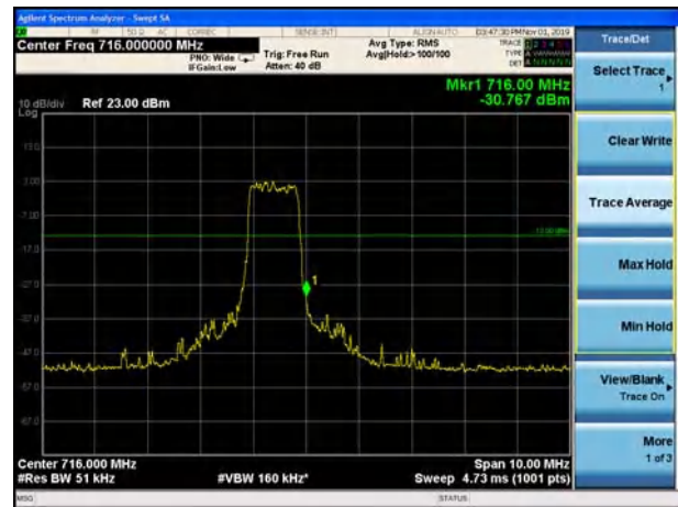
LTE Band 12 16QAM 3MHz CH-High, 1 RB
