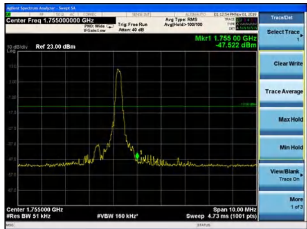
LTE Band 4 16QAM 10MHz CH-High, 100%RB
