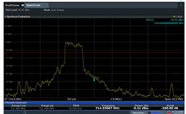
LTE Band 85 16QAM 10MHz CH-High, 100%RB
