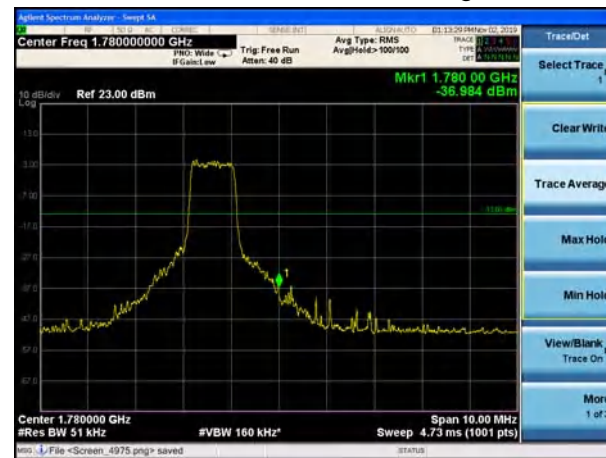
LTE Band 66 16QAM 20MHz CH-High, 1 RB
