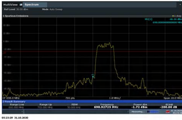
LTE Band 85 16QAM 10MHz CH-Low, 1 RB
