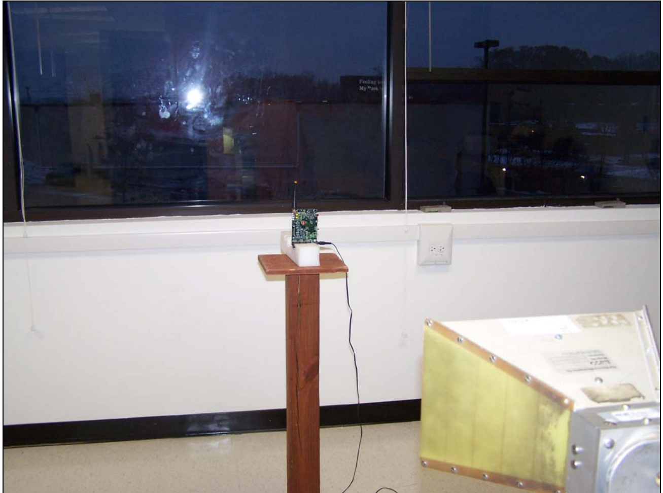
Photograph 13. Band Edge and Spurious Radiated Emissions Test Setup
