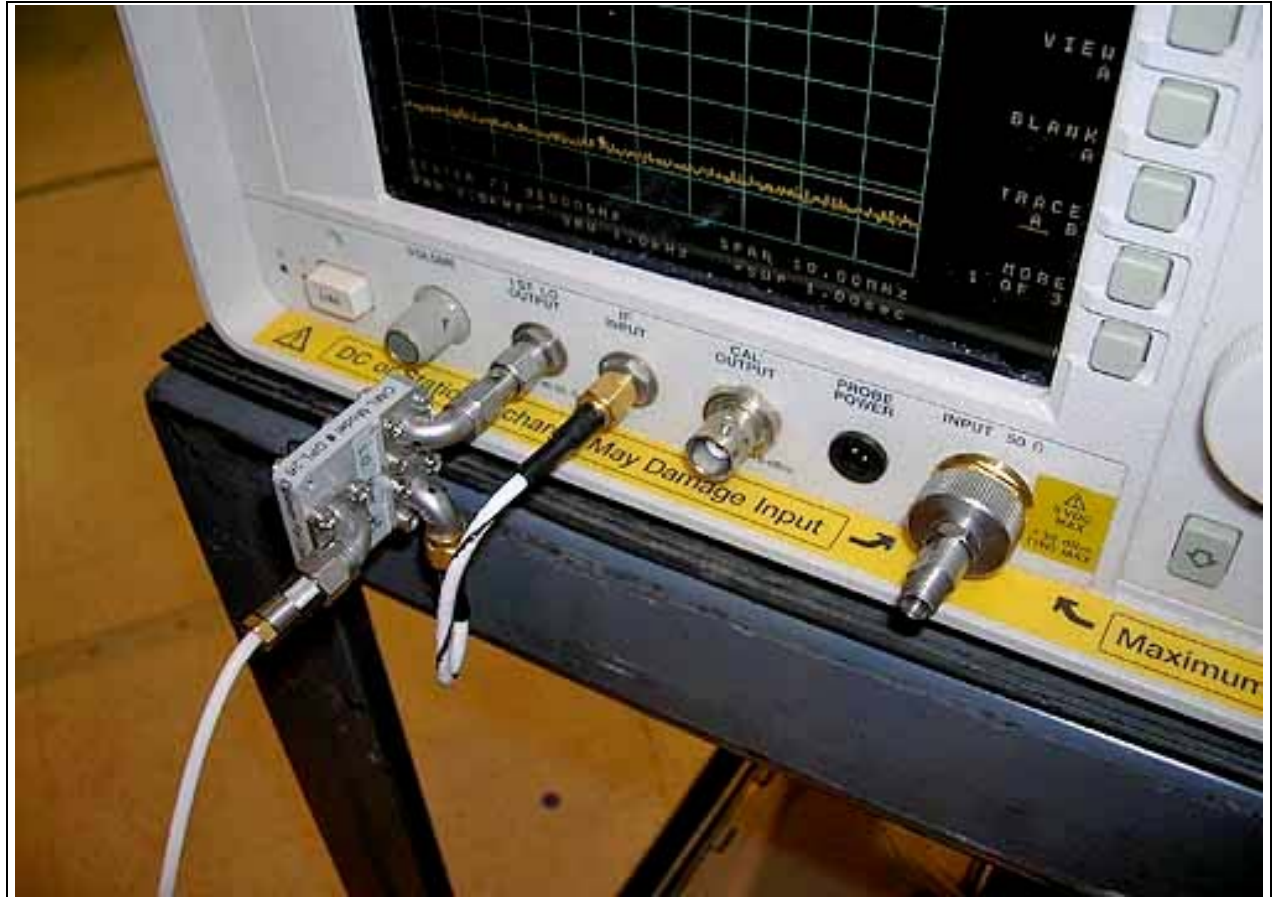
40-100 GHz Setup - Diplexer installed on SA
