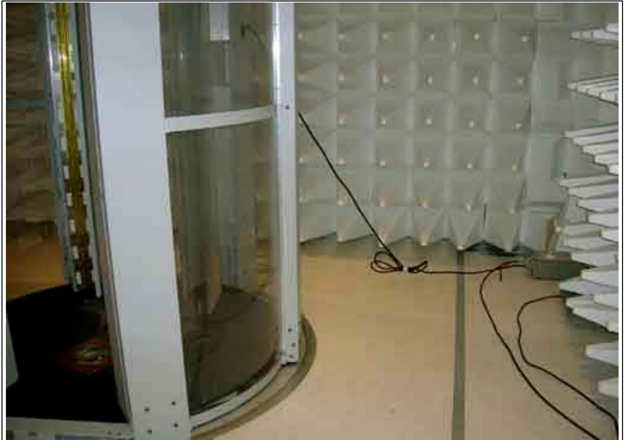
Mains Conducted Emissions - Front View
