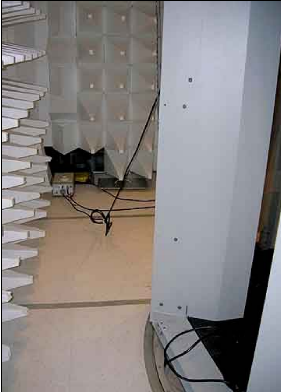
Mains Conducted Emissions - Side View
