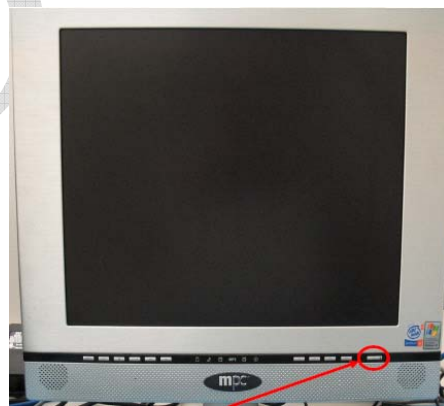
Figure 3 Operator Console power switch
