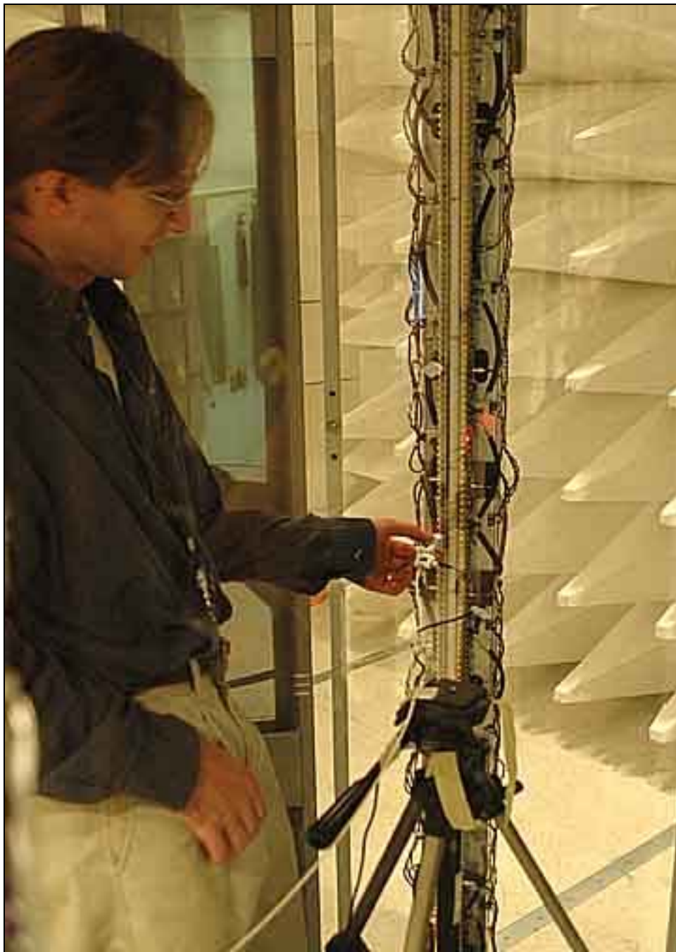
Radiated Emissions - 40-100 GHz Sample Setup Using Mixers
