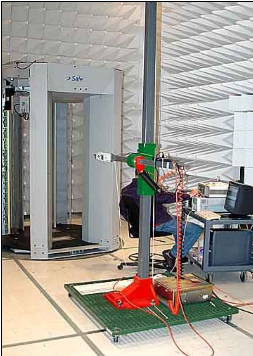
Radiated Emissions - 12-40 GHz Sample Setup at 1 Meter
