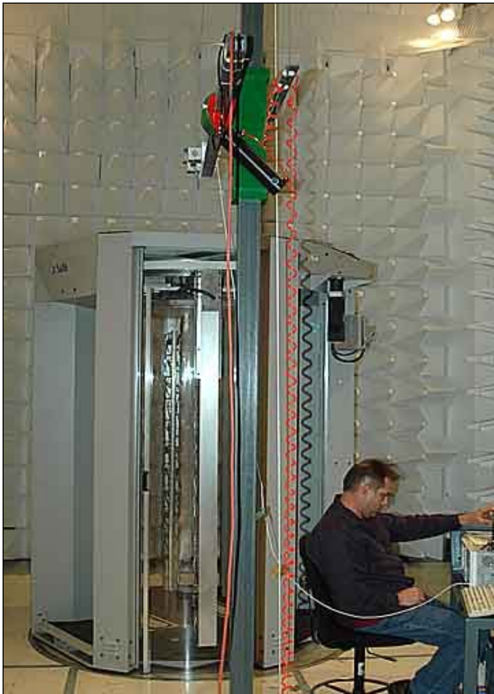
Radiated Emissions - 12-40 GHz Sample Setup at 3 Meters
