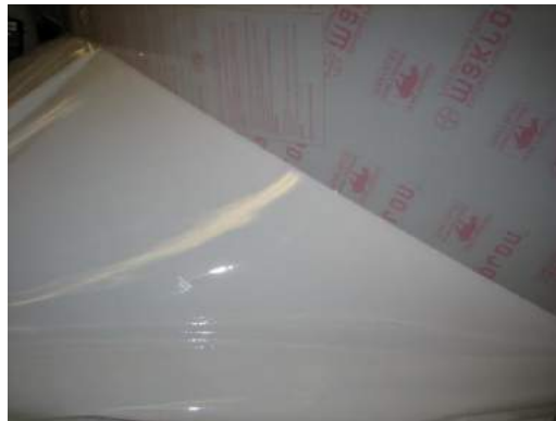
Figure 83: Scratch Guard Film Being Removed
