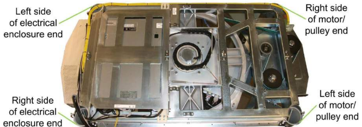
Figure 69: Cabling Route with Power Input Box, OCP, and Other Cables Together
