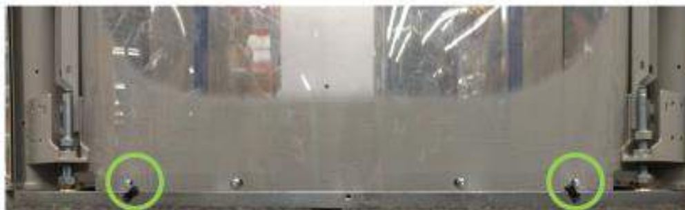
Figure 43: U-clip Installed on Frame
