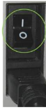
Figure 52: Power Switch in the On Position
