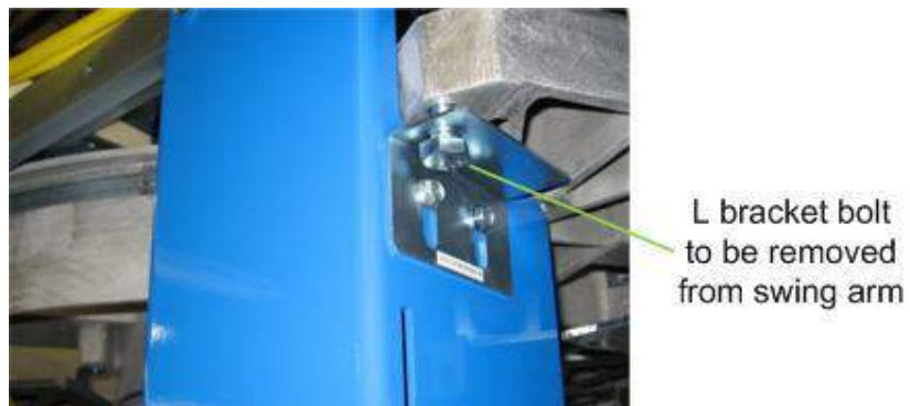
Figure 40: Bolt Through L Bracket into Swing Arm
