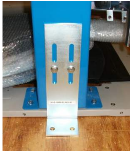
Figure 7: Screws/Bolts and Brackets to Be Removed
