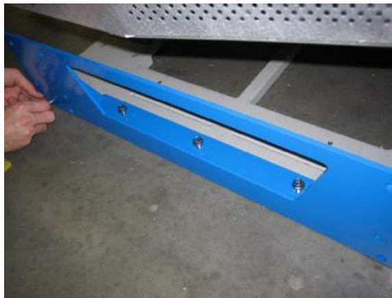
Figure 21: Caster End Plate Installation
