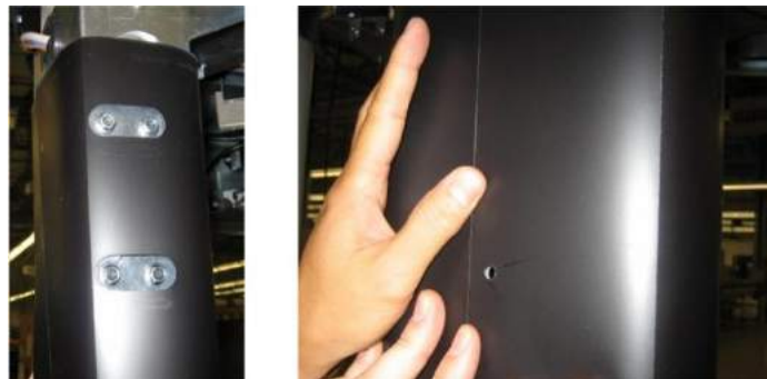
Figure 59: Cosmetic Mast Wrap Installation
