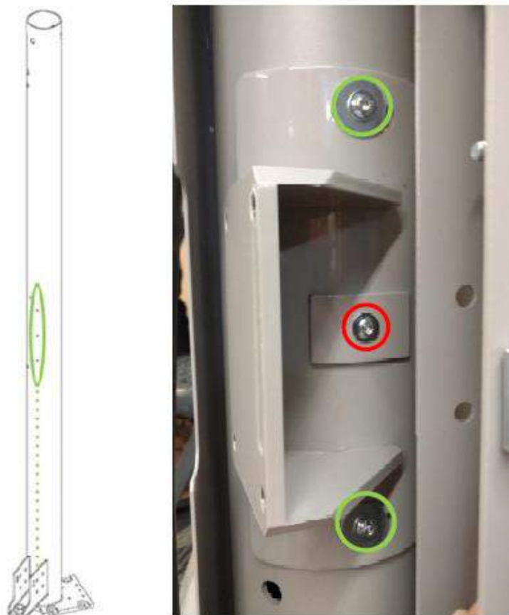
Figure 48: Mounting Bracket Installed on Column
