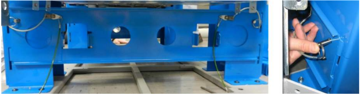
Figure 26: Lifting Bracket with Quick-Release Pin Being Inserted
