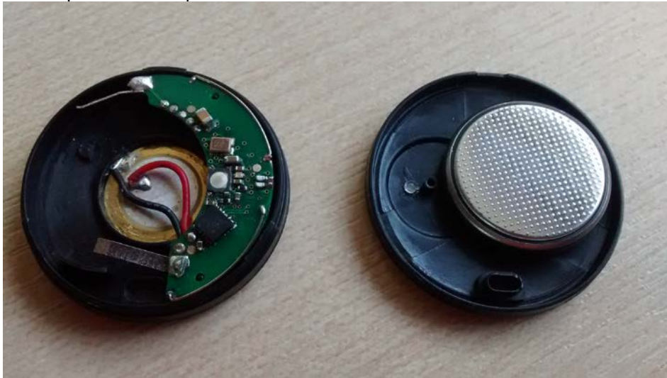
Case Open – PCB Top side
