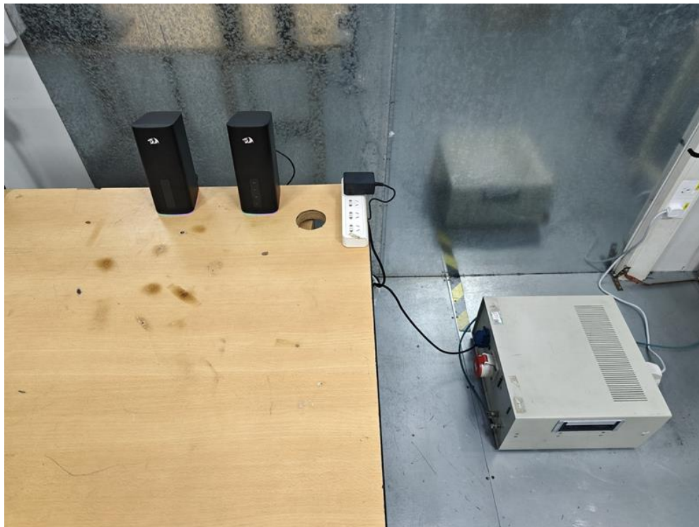
Conducted Emission Test Setup:
