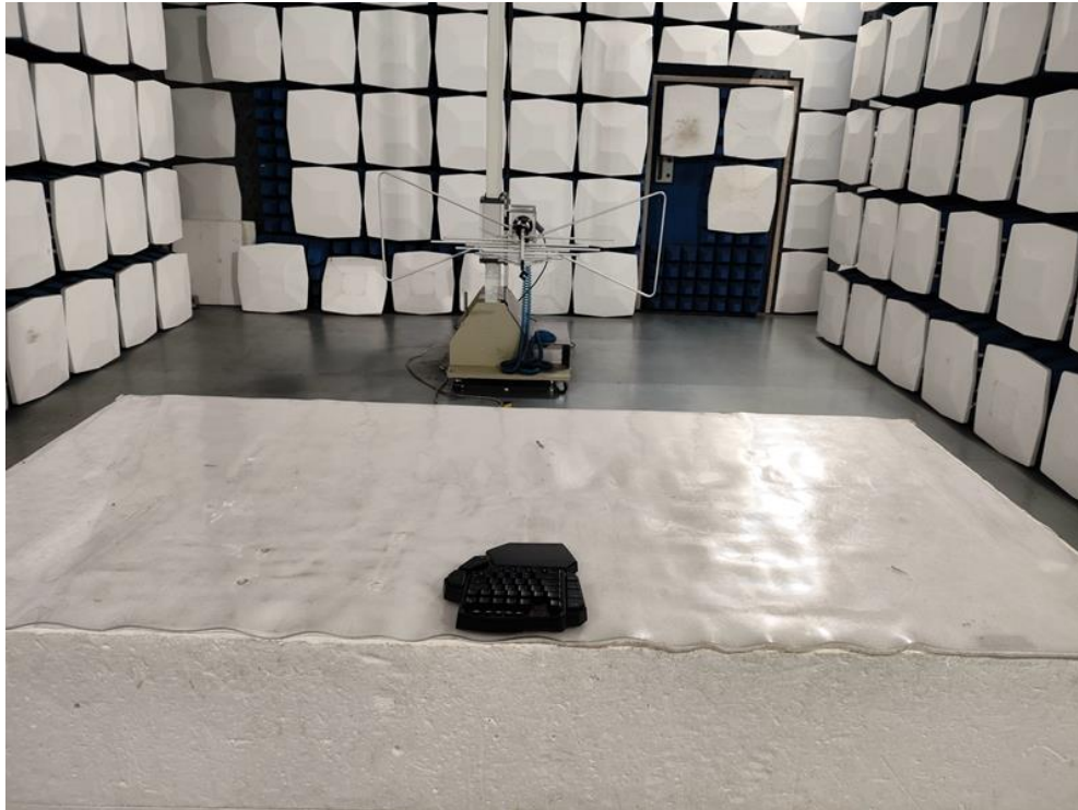
Radiated Emission Test Setup:
