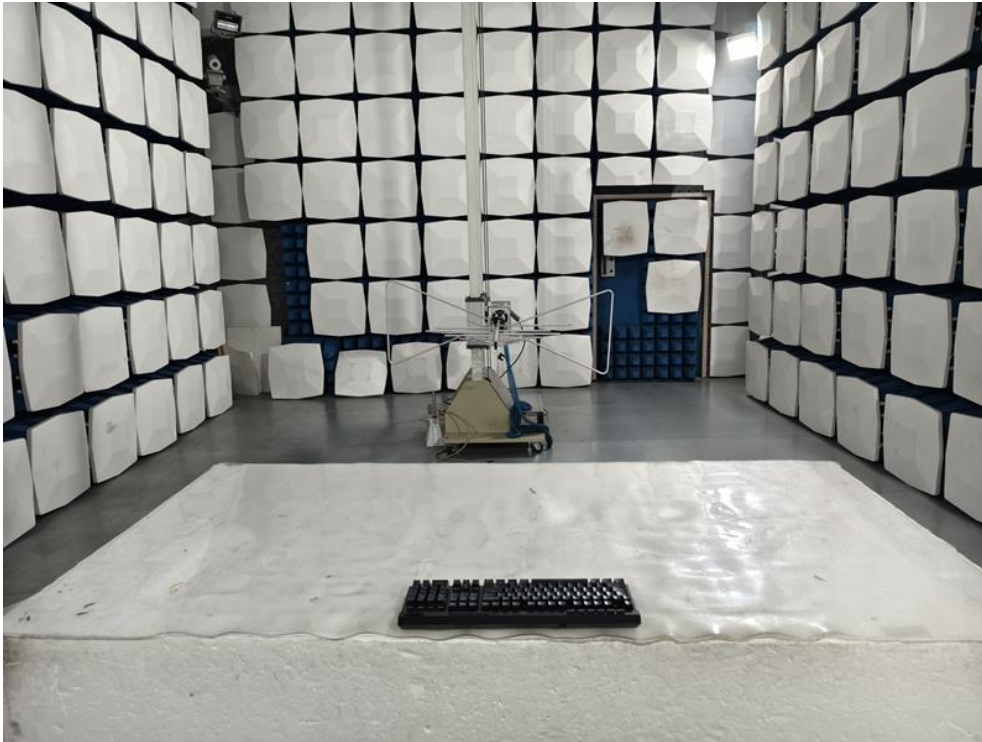
Radiated emission test view
