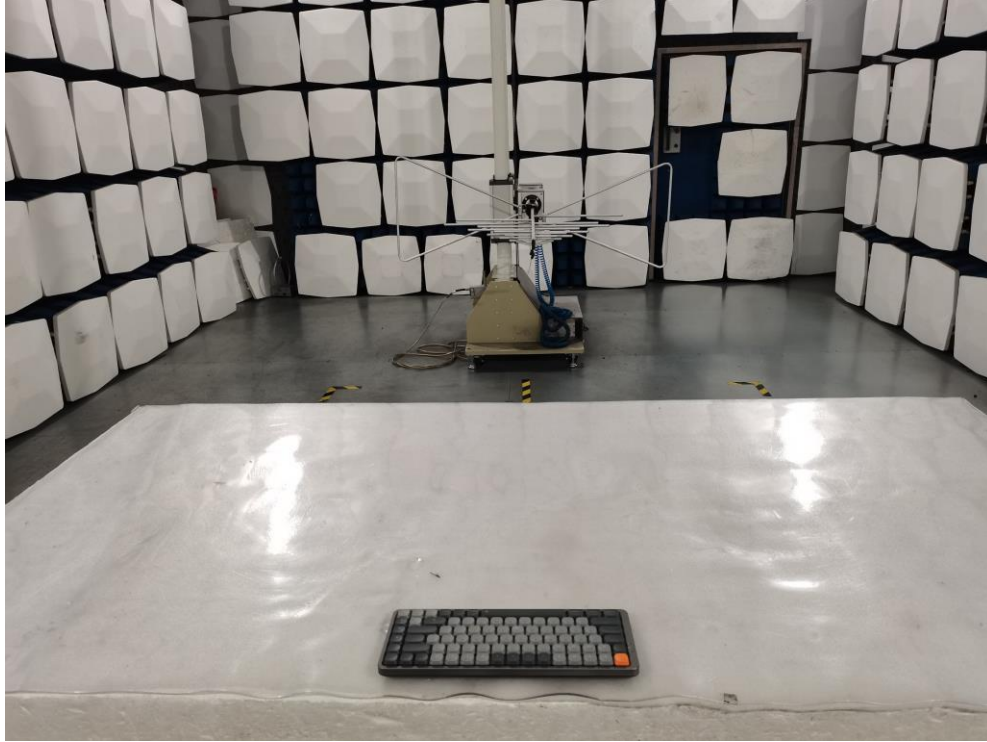
Radiated Emission Test Setup:
