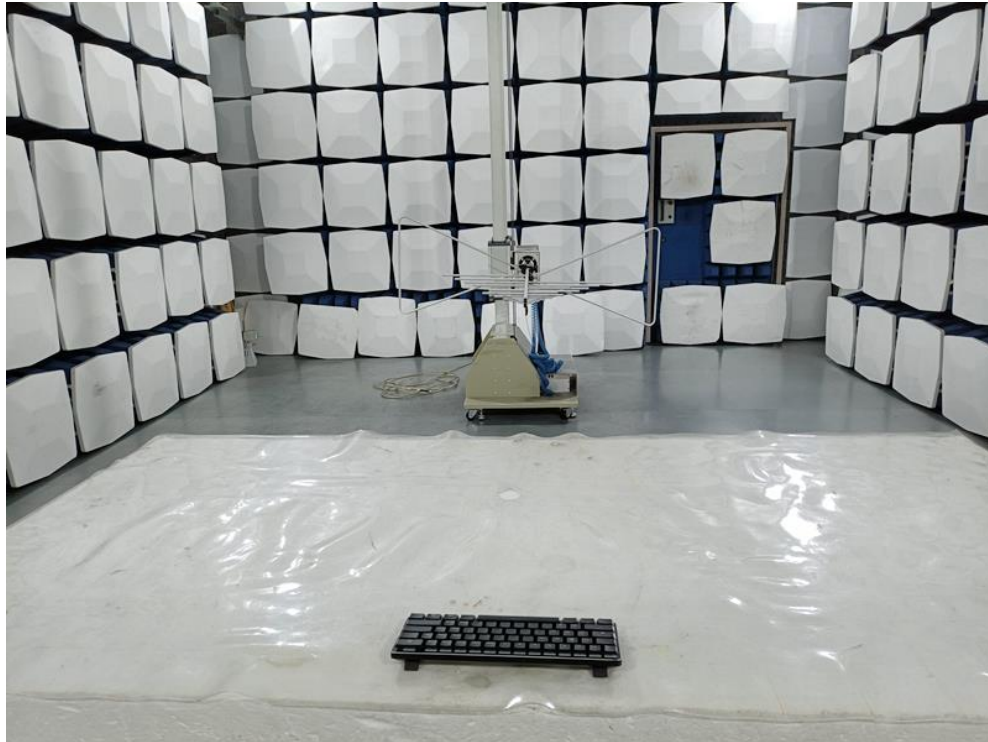
Radiated Emission Test Setup:
