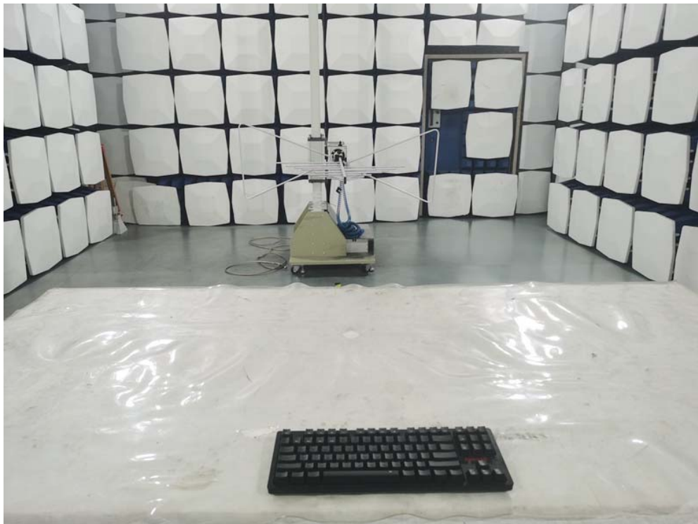
Radiated emission test view
