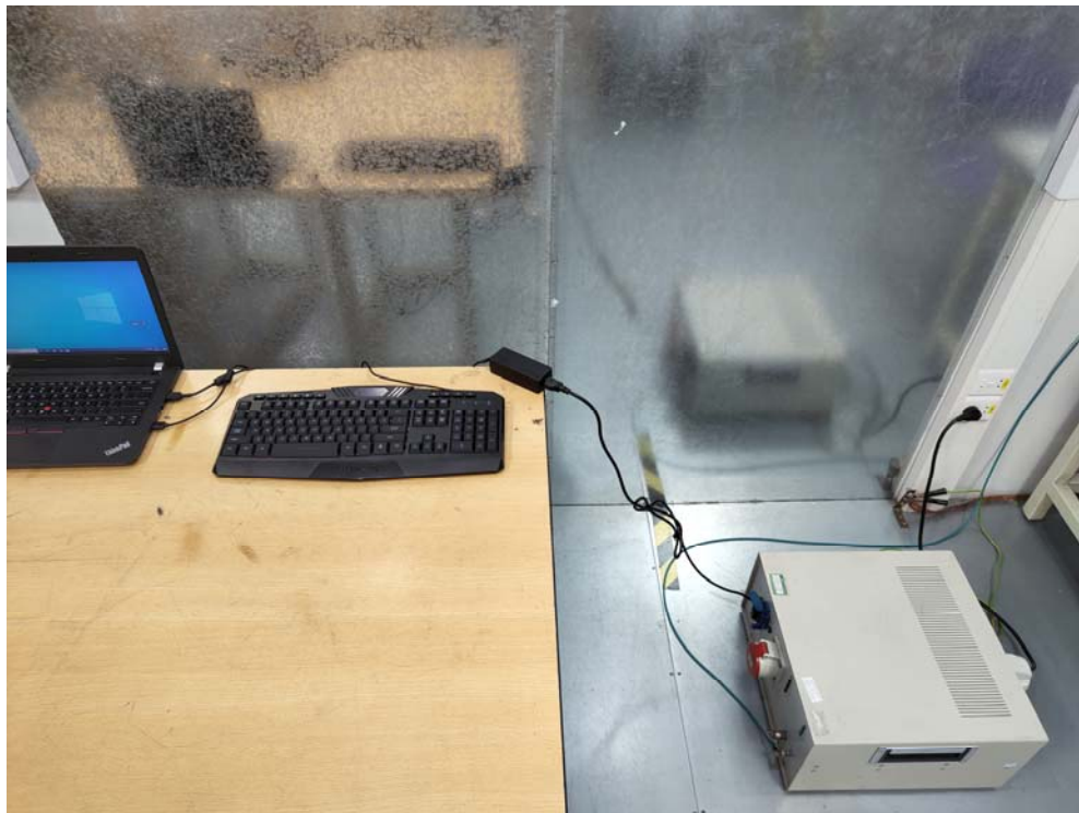
Conducted Emission Test Setup:
