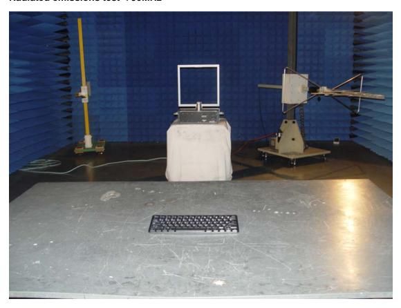
Radiated emissions test 30MHz-1GHz
