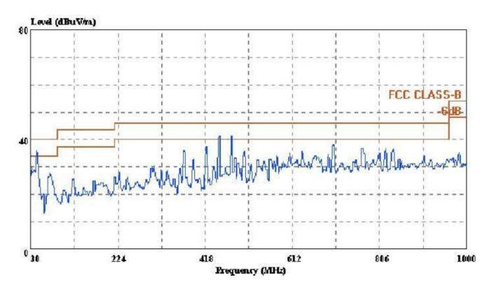
Condition: FCC CLASS-B 3m ATC VULB9163(NEW) VERTICAL
