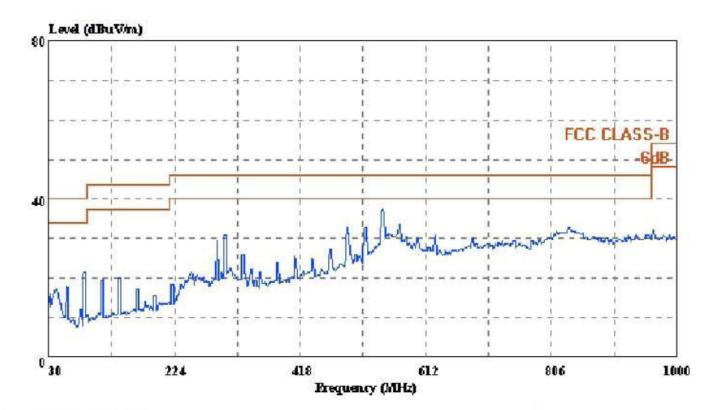
Condition: FCC CLASS-B 3m ATC VULB9163(NEW) VERTICAL
