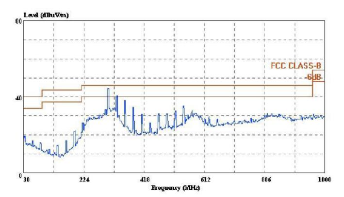
Condition: FCC CLASS-B 3m ATC VULB9163 (NEW) HORIZONTAL
