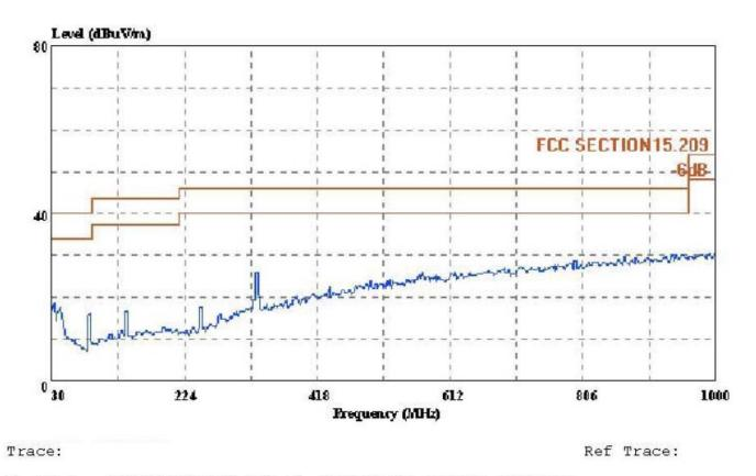
Condition: FCC SECTION15.209 3m ATC FCC15C ANTENNA VERTICAL eut : Wired&Wireless Mouse m/n:DS-2135-Z power : DC 2.4V memo : TX manuf : Eastern Times sample no.: 063231
