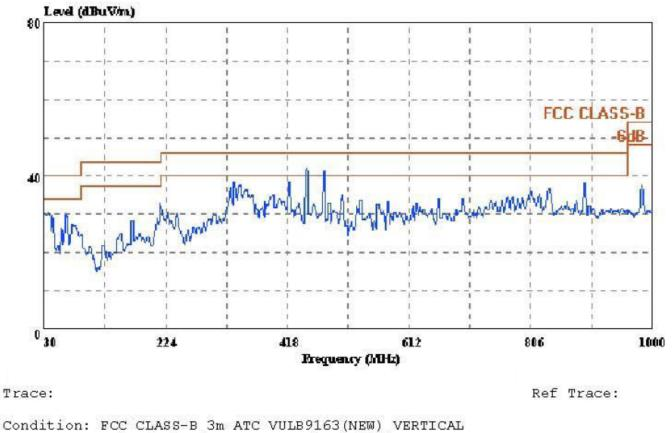
Condition: FCC CLASS-B 3m ATC VULB9163(NEW) VERTICAL eut : Wired&Wireless Mouse m/n:DS-2135-Z power : USB 5.0V memo : CONNECT TO PC manuf : Eastern Times sample no.: 063231
