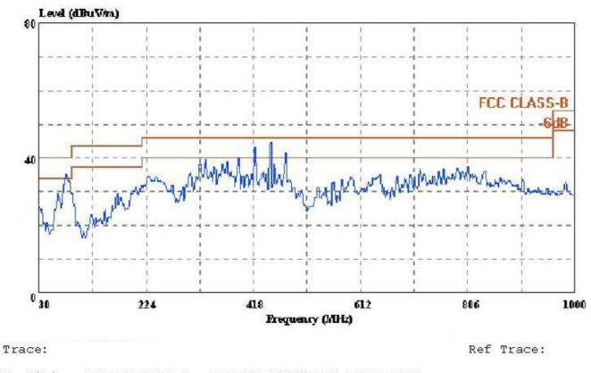
Condition: FCC CLASS-B 3m ATC VULB9163(NEW) HORIZONTAL eut : Wired&Wireless Mouse m/n:DS-2135-Z power : USB 5.0V memo : CONNECT TO PC manuf : Eastern Times sample no.: 063231
