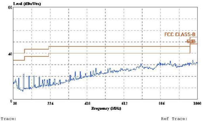
Condition: FCC CLASS-B 3m ATC VULB9163(NEW) VERTICAL eut : Wireless Optical Mouse power : DC 2.4V memo : TX manuf : Eastern Times sample no.: 071961 : m/n:DS-2060(2060-F+2068-D)
