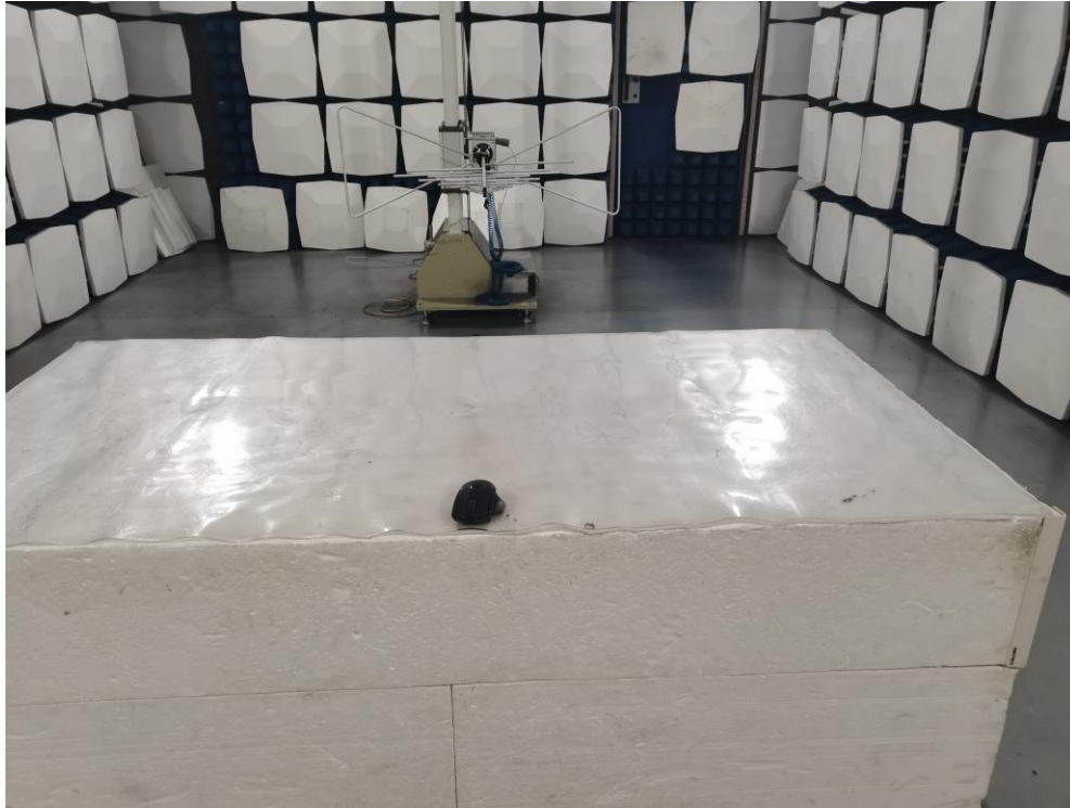
Radiated Emission Test Setup:
