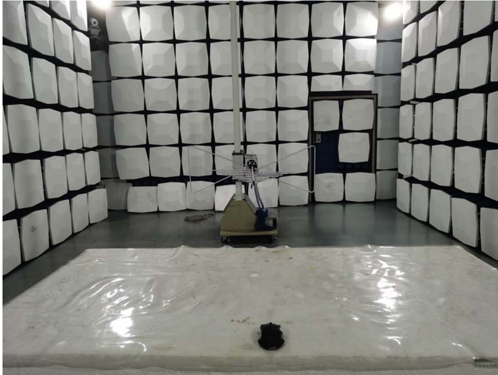
Radiated Emission Test Setup:
