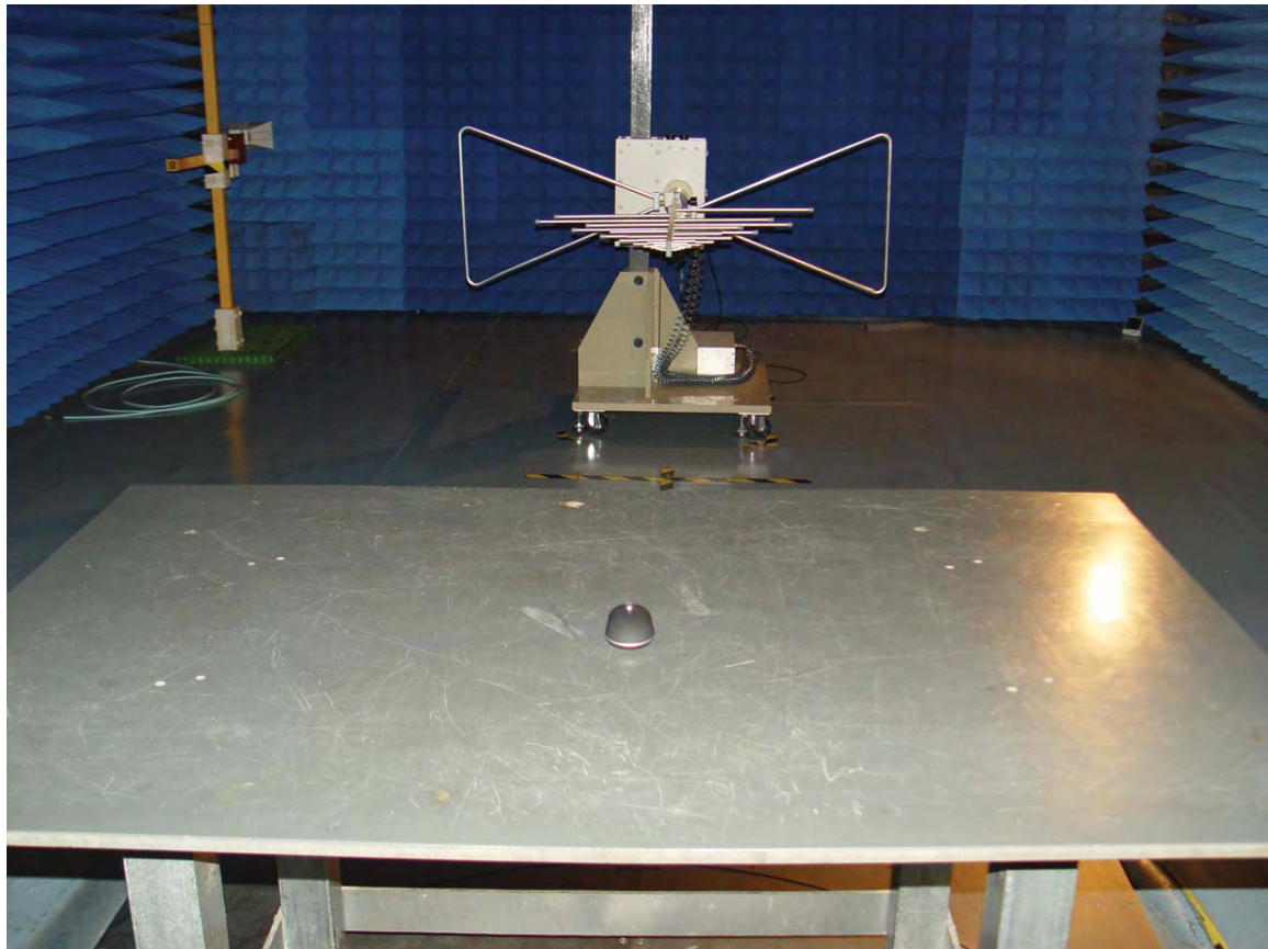
Radiated emissions test < 1GHz
