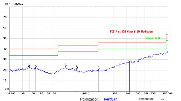
Site Polarization: Vertical Temperature: 25 Limit: FCC Part 15B Class B 3M Radiation Power: DC 1.5V Humidity: 55 %
