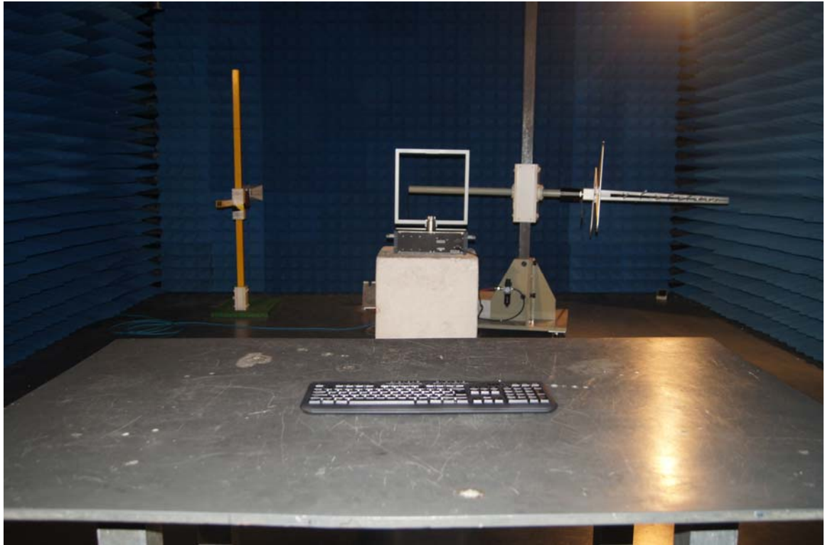
Radiated emissions test < 30MHz
