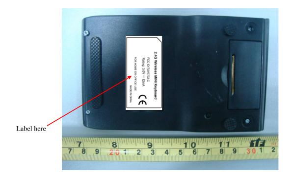
The label shown shall be permanently affixed at a conspicuous location on the device and be readily visible to the user at the time purchase (FCC requirements per §2.925)
