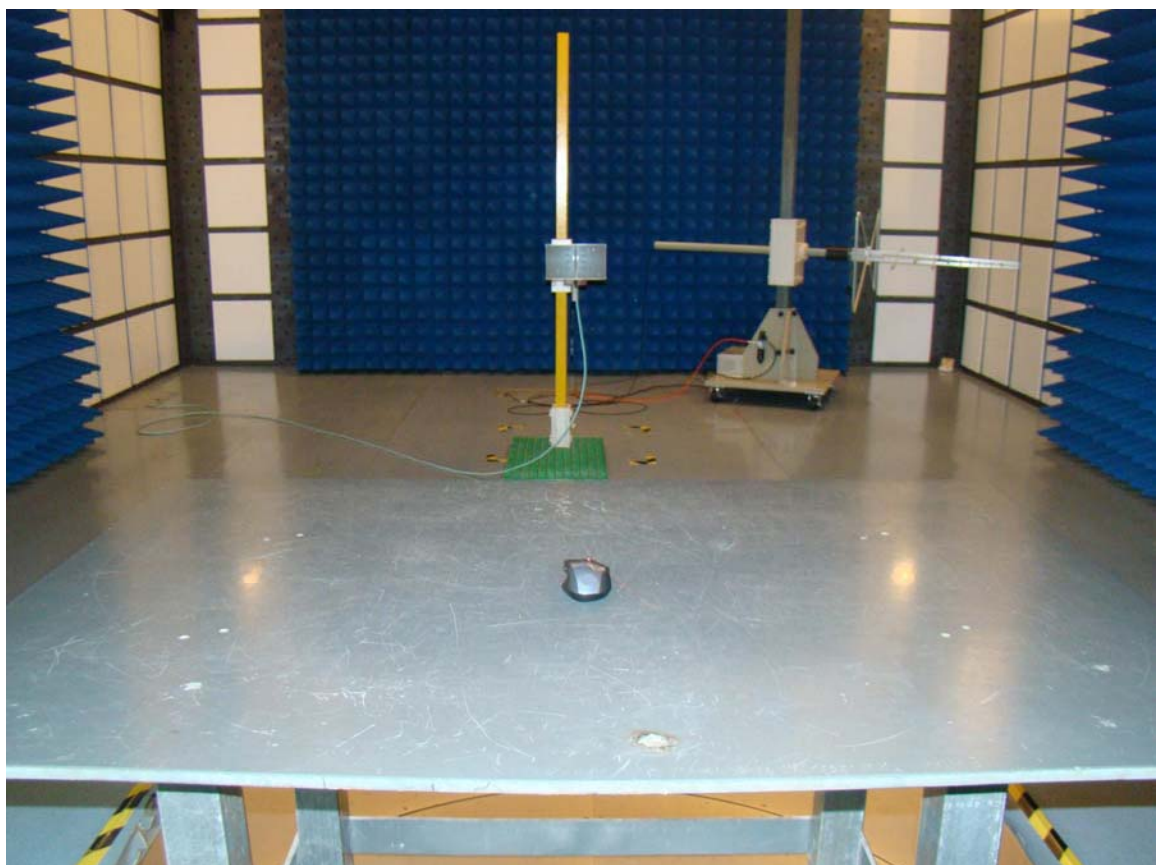
Radiated emissions test > 1GHz
