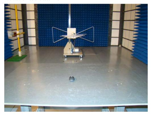
Radiated emissions test > 1GHz
