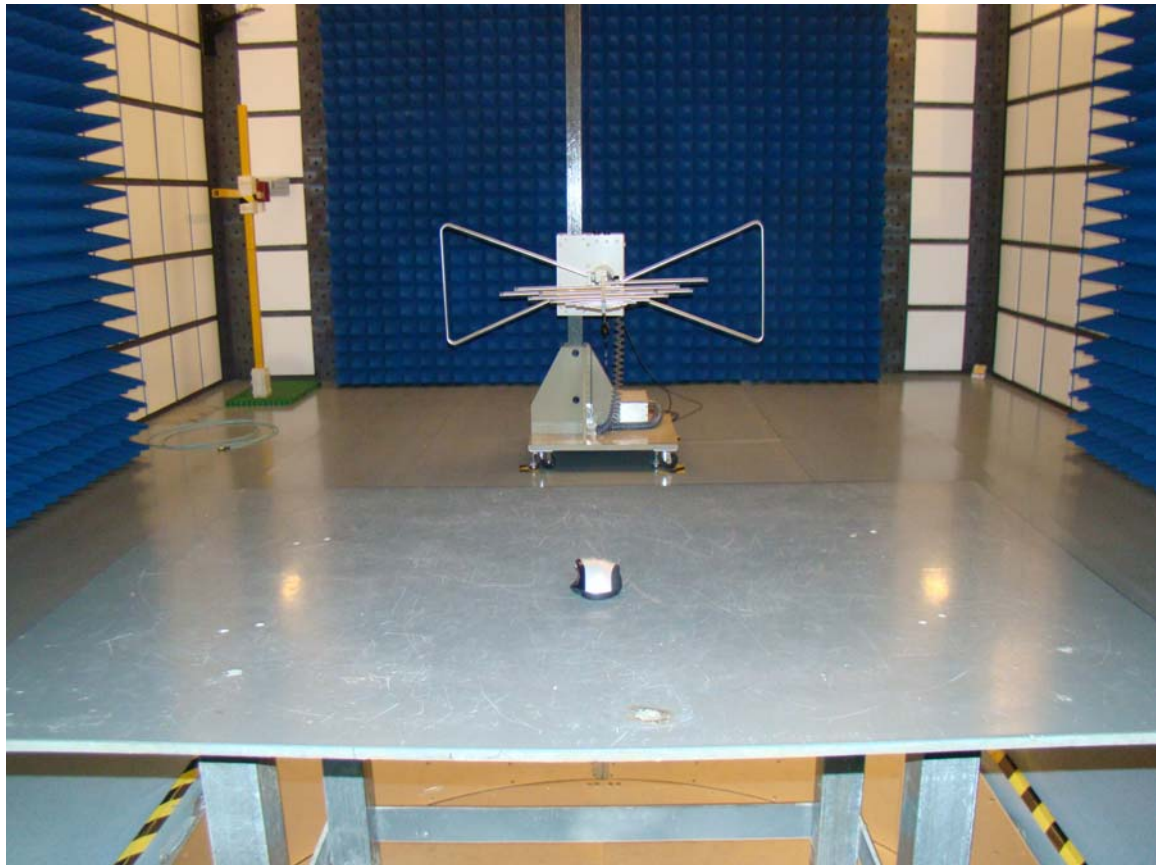
Radiated emissions test < 1GHz
