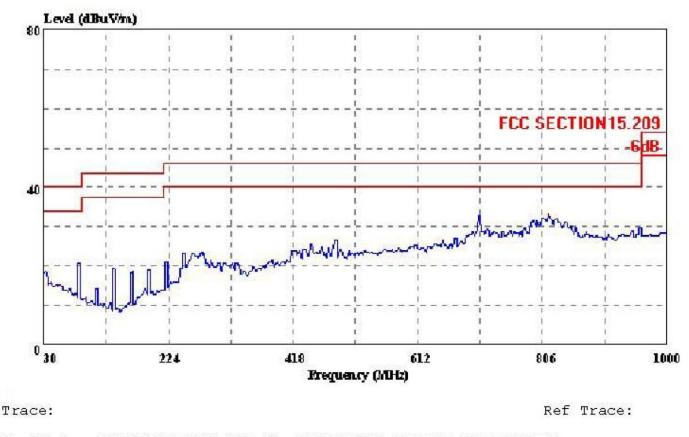
Condition: FCC SECTION15.209 3m ATC FCC15C ANTENNA HORIZONTAL eut : Wireless Optical Mouse : M/N:DS-2135(2135-L+2121-L) power : DC 2.4V memo : TX manuf : Eastern Times sample No.: 080547 report No.: ATE20080335
