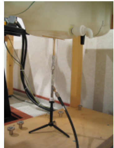
Photo of the dipole Antenna
