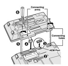
IP8800 Series Expansion Modules Quick Installation Guide
