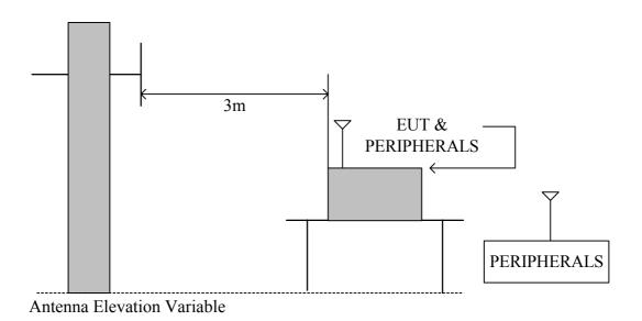
The diagram below shows the test setup that is utilized to make the measurements for emission above 1GHz.
