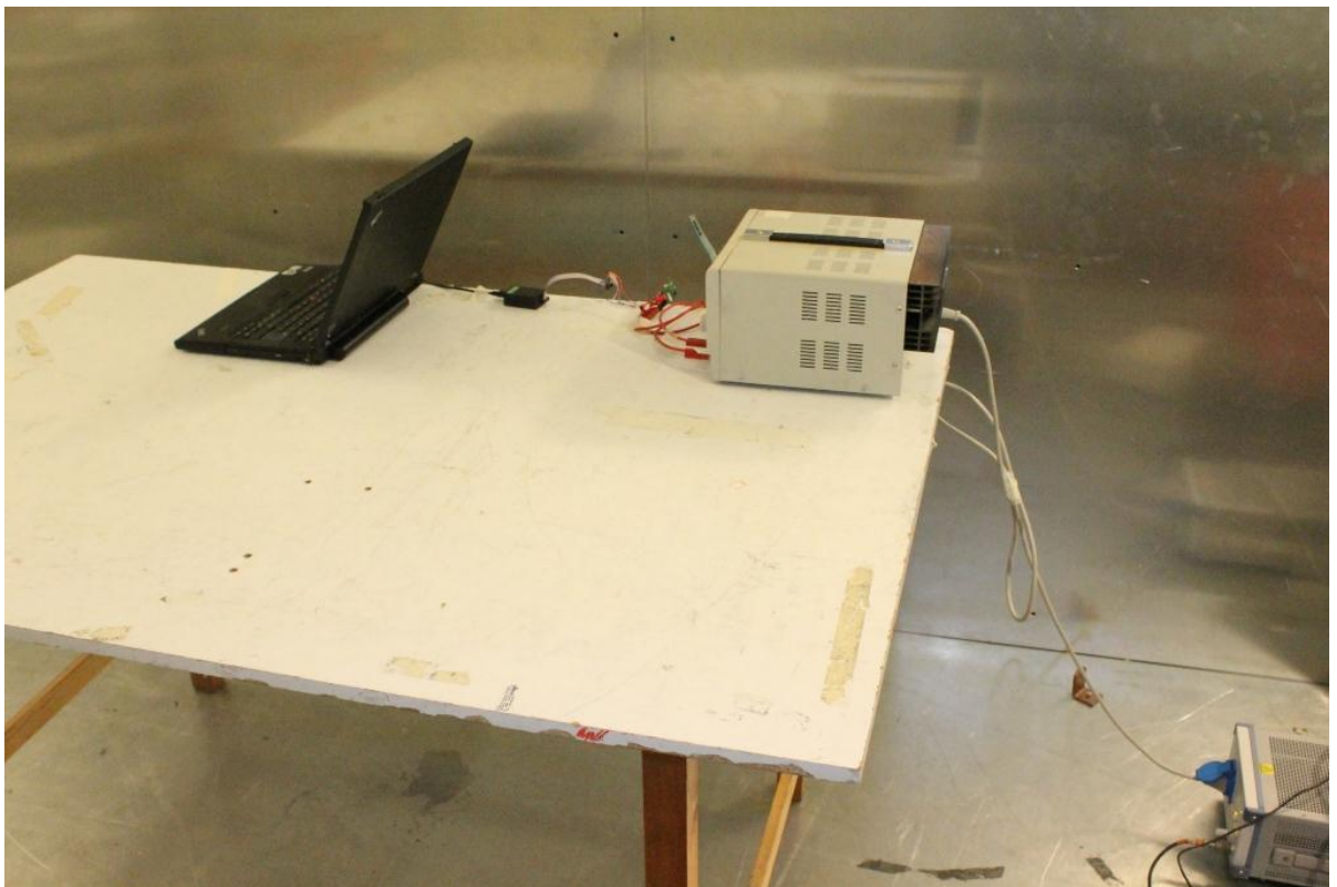
Photograph 2. AC power line conducted emissions test setup
