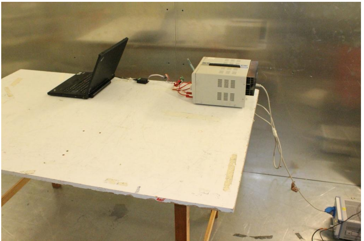
Photograph 2. AC power line conducted emissions test setup
