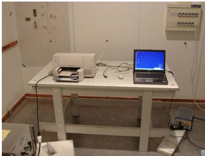
Picture 4: Conducted emission measurement setup
